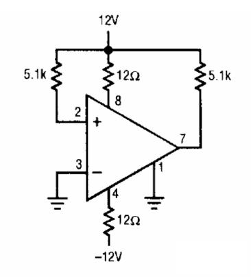
Figure A.1. Irradiation bias drawing for the units to be irradiated under electrical bias. This figure was extracted from LINEAR TECHNOLOGY CORPORATION, Drawing Number: 05-08-5012 REV. L "MICROCIRCUIT, LINEAR, MFG RH1011, VOLTAGE COMPARATOR".
