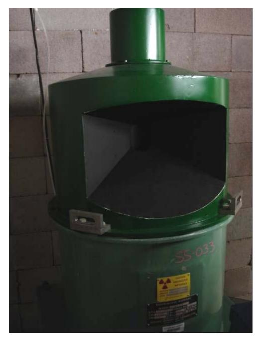
Figure 2.1. Radiation Assured Devices' Co-60 irradiator. The dose rate is obtained by positioning the deviceunder-test at a fixed distance from the gamma cell. The dose rate for this irradiator varies from approximately 50rad(Si)/s close to the rods down to <1mrad(Si)/s at a distance of approximately 4-meters.
