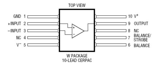
Figure B.2. W package drawing (for reference only). This figure was extracted from LINEAR TECHNOLOGY CORPORATION RH1011 Datasheet.
