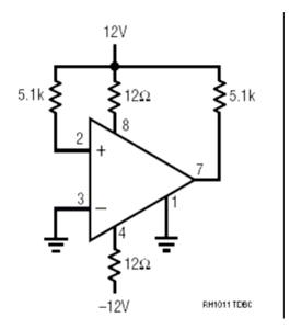
Figure B.1. Irradiation bias drawing for the units to be irradiated under electrical bias. This figure was extracted from LINEAR TECHNOLOGY CORPORATION RH1011 Datasheet. Pin numbers are for the H or J8 package.
