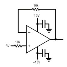
Figure B.1. Irradiation bias drawing for the units to be irradiated under electrical bias. This figure was extracted from the LINEAR TECHNOLOGY CORPORATION RH1014M Quad Precision Operational Amplifier Datasheet.
