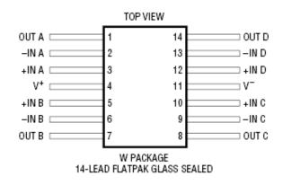
Figure B.2. Package drawing (for reference only). This figure was extracted from the LINEAR TECHNOLOGY CORPORATION RH1014M Quad Precision Operational Amplifier Datasheet.
