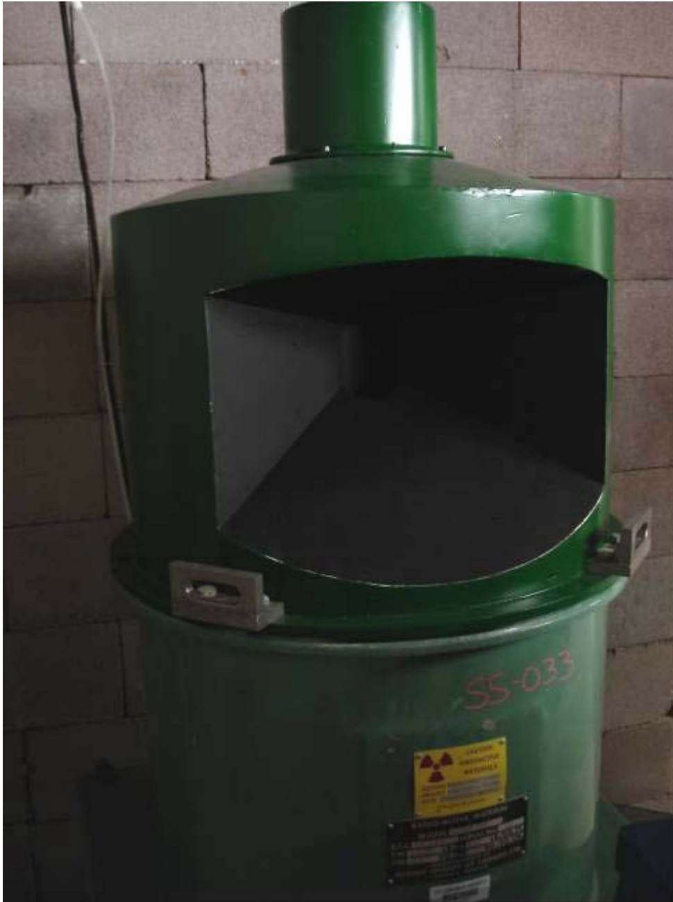
Figure 2.1. Radiation Assured Devices' Co-60 irradiator. The dose rate is obtained by positioning the device-under-test at a fixed distance from the gamma cell. The dose rate for this irradiator varies from approximately 50rad(Si)/s close to the rods down to <1mrad(Si)/s at a distance of approximately 4-meters.
