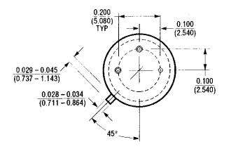
NOTE: 1. FOR SOLDER DIP LEAD FINISH, LEAD DIAMETER IS  $\frac{0.016-0.024}{(0.406-0.610)}$
