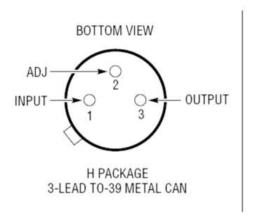
Figure B.2. H package drawing (for reference only). This figure was extracted from the LINEAR TECHNOLOGY CORPORATION RH117 Datasheet.
