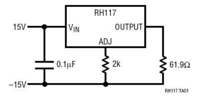
Figure B.1. Irradiation bias drawing for the units to be irradiated under electrical bias. This figure was extracted from LINEAR TECHNOLOGY CORPORATION, RH117 Datasheet.
