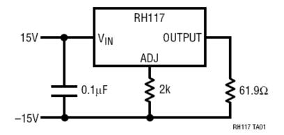
Figure B.1. Irradiation bias drawing for the units to be irradiated under electrical bias. This figure was extracted from LINEAR TECHNOLOGY CORPORATION, RH117 Datasheet.
