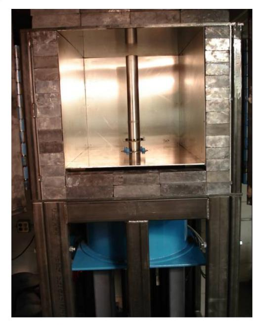
Figure 2.1. Radiation Assured Devices' high dose rate Co-60 irradiator. The dose rate is obtained by positioning the device-under-test at a fixed distance from the gamma cell. The dose rate for this irradiator varies from approximately 120rad(Si)/s close to the rods down to 1rad(Si)/s at a distance of approximately 2-feet.
