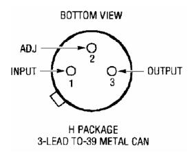
Figure B.2. H package drawing (for reference only). This figure was extracted from the LINEAR TECHNOLOGY RH117 Datasheet.
