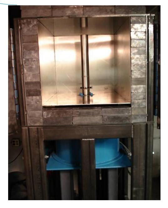
Figure 2.1. Aeroflex RAD's high dose rate Co-60 irradiator. The dose rate is obtained by positioning the device-under-test at a fixed distance from the gamma cell. The dose rate for this irradiator varies from approximately 300rad(Si)/s close to the rods down to 1rad(Si)/s at a distance of approximately 2-feet.
