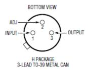
Figure B.2. H Package drawing (for reference only). This figure was extracted from Linear Technology RH117 Datasheet I.D No. 66-11-0135 Revision C.
