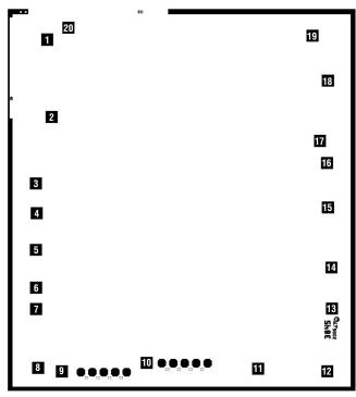
113mils × 124mils, Backside metal: Alloyed Gold Layer Backside potential: GND
