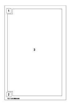
157mils × 102mils<sup>2</sup>, Backside metal: Alloyed Gold Layer Backside potential: NMOS Drain
