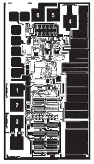
57mils × 33mils, 12mils thick. Backside metal: Gold Backside potential: V<sup>-</sup>
