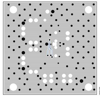
Figure 8. Layer 2 (Ground Plane)
