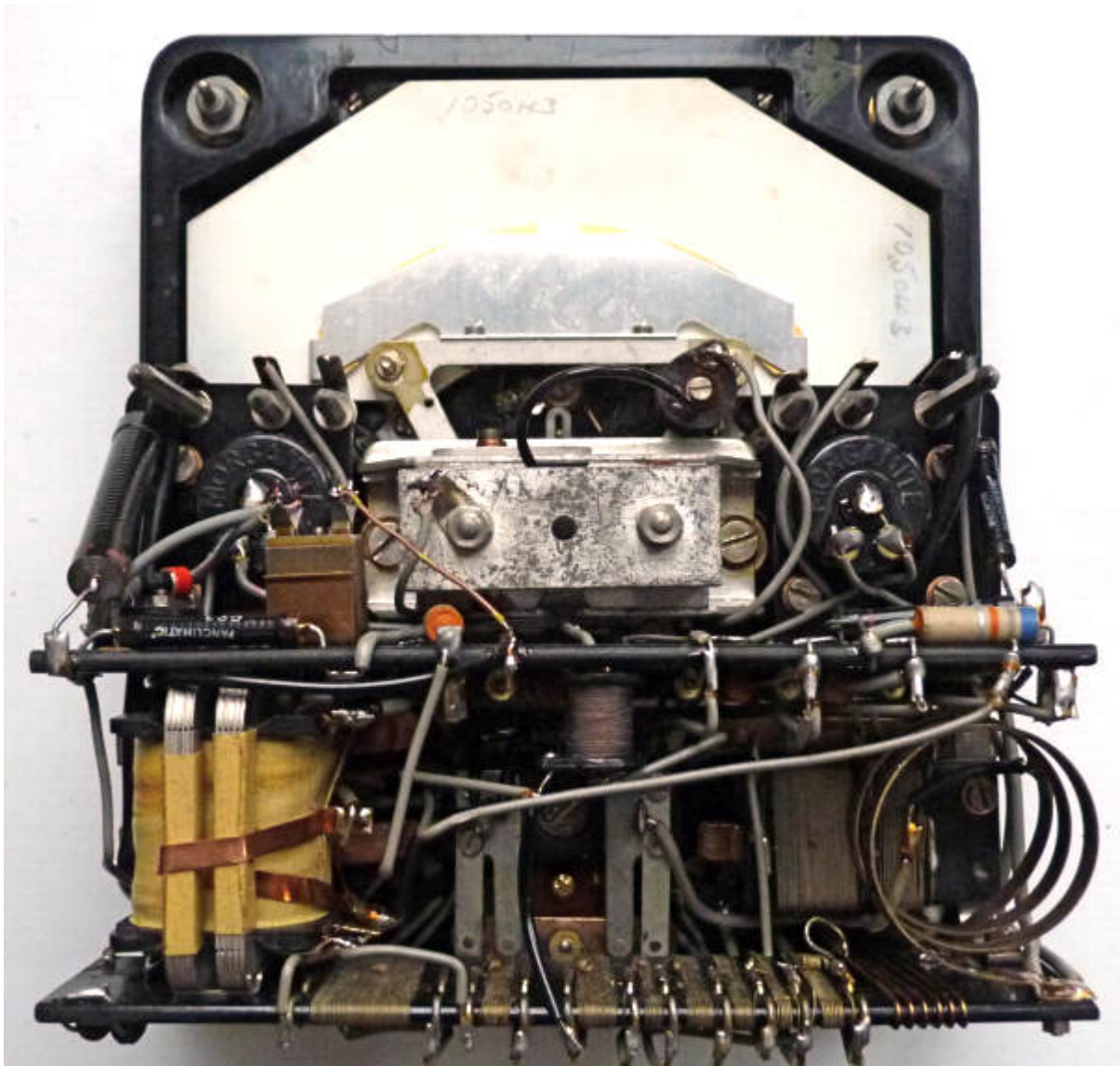
AVO Model8 MkII interior (the rectifier is not original)
