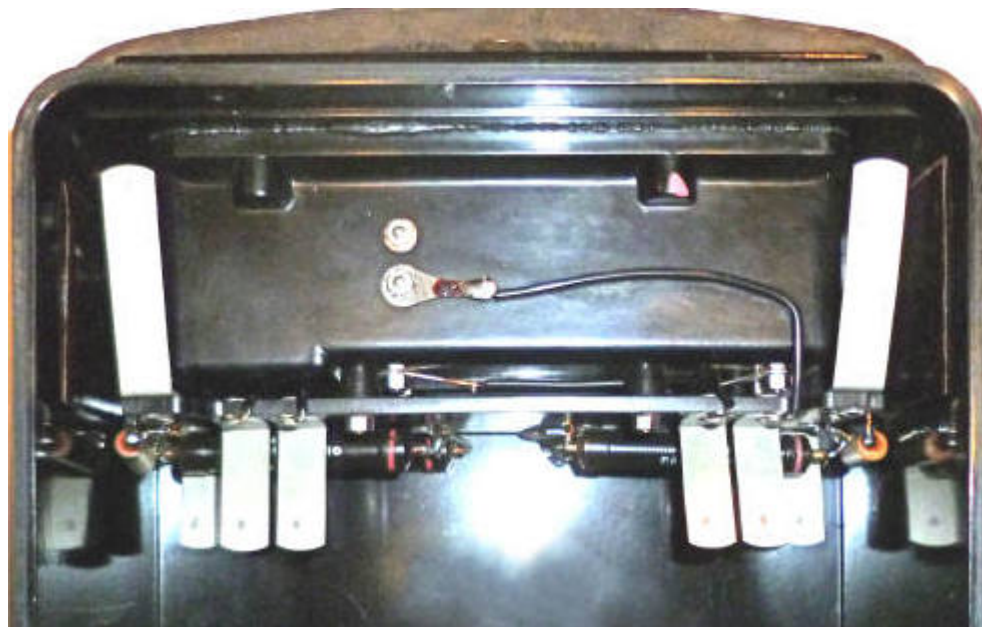
AVO Model8 battery and high voltage contact leaf springs. [The four inner ones are for the batteries]
