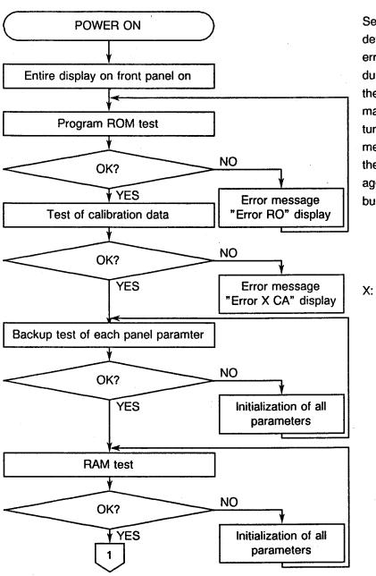
See section 5.2 for POWER ON details of error messages. If error message display occurs during this power-on procedure, the R6871E/E-DC is malfunctioning. In such cases, turn the power off with the error message left on the display and then contact the sales division or agency nearest your place of business.
