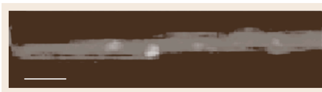
Fig. 5.106 STEM-EELS image of Gd (white) atoms in a carbon (gray) nanotube. Scale bar = 3 nm. After [5.81]
