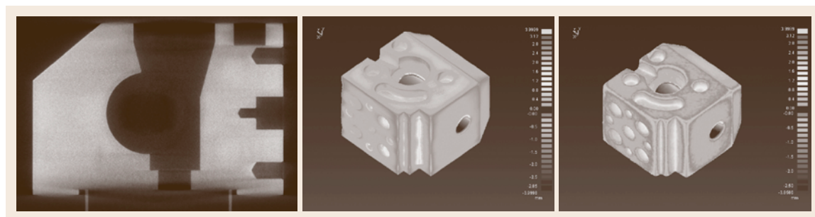
Fig. 16.63 Test sample of aluminum ( \varnothing about 100 mm). The image ( left ) shows a cross section of the measurement with the 320-kV equipment (320-kV x-ray: 220 kV, 100 μA; prefilter: 1.5 mm Sn; projections: 900/360°; exposure time: 2.28 s per projection; voxel: (0.12 mm 3 ); matrix: 1023 × 1023 × 605). The image ( middle ) shows the deviation against the CAD data and the image ( right ) the deviation against the measurement with LINAC (10.5 MeV, 20 Gy; prefilter: 90 mm Fe; projections: 720/360°; exposure time: 0.8 s per projection; voxel: (0.65 mm 3 ); matrix 255 × 255 × 201)
