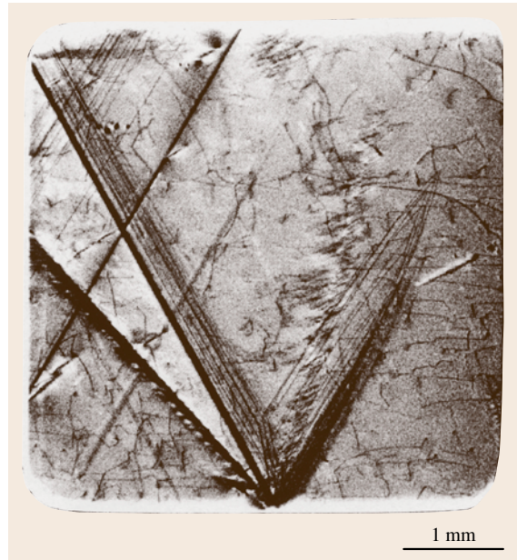
Fig. 5.78 An anomalous transmission x-ray topographic image of dislocations in GaAs introduced by plastic deformation. The sample thickness is 0.5 mm (Courtesy of Dr. I. Yonenaga)
