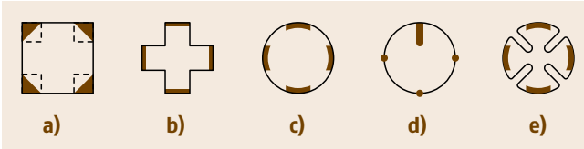
Fig. 9.38a–e van der Pauw test samples with nonideal finite contact sizes (after [9.44])
