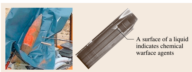
Fig. 16.53 Inspection of a grenade of World War I, filled with chemical warfare. The chemical agent can be detected, by visualization of the liquid-level line inside the grenade
