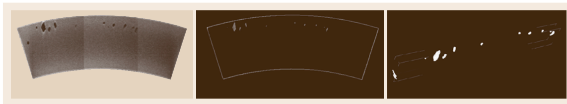
Fig. 16.65 Electron beam welding of a section (size 40 \times 100 \times 300 mm) of a Cu canister. The image (left) shows a cross section containing the flaws, flaws after segmentation (middle) projected into a plane and the flaws after conversion to the STL data format (right). Source: LINAC 10.5 MeV, 15 Gy; prefilter: 90 mm Fe; projections: 720/360^\circ ; exposure time: 0.2 s per projection; voxel: (0.653 \text{ mm}^3) ; matrix: 255 \times 255 \times 532
