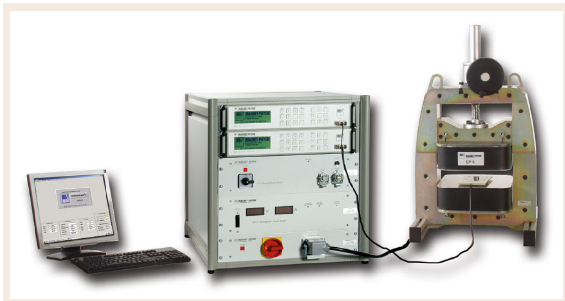
Fig. 10.2 Hysteresisgraph for hard magnetic materials. The cabinet contains two fluxmeters for H and J measurement and the electromagnet power supply. The specimen and surrounding coil are placed between the poles of the electromagnet (Permagraph C Magnet-Physik Dr. Steingroever GmbH, Köln)
