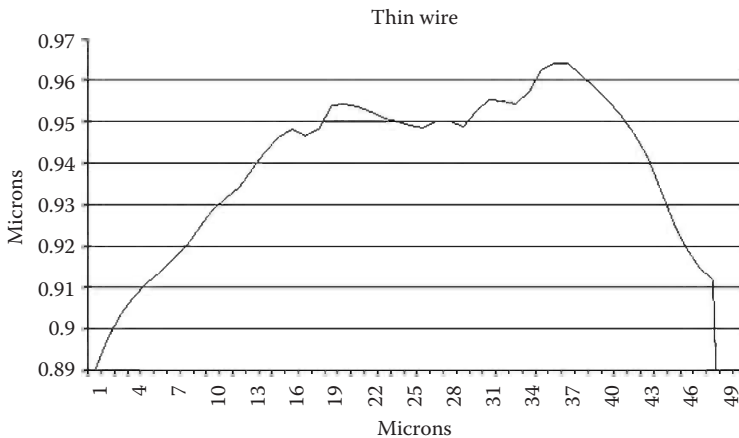
FIGURE 11.8 A thin wire, scanned with a conoscopic probe with a focus spot comparable to the wire thickness. At the peak, the curvature is not correctly captured.
