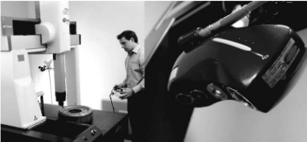
FIGURE 6.8 Left: CMM. Right: 3D laser scanner mounted on a CMM.
