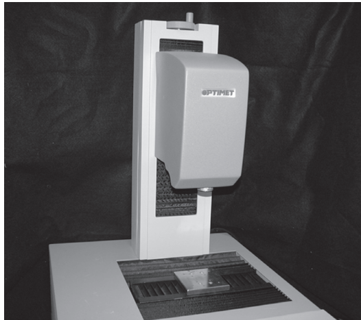
FIGURE 11.5 Scanning system using a conoscopic sensor made by Optimet.
