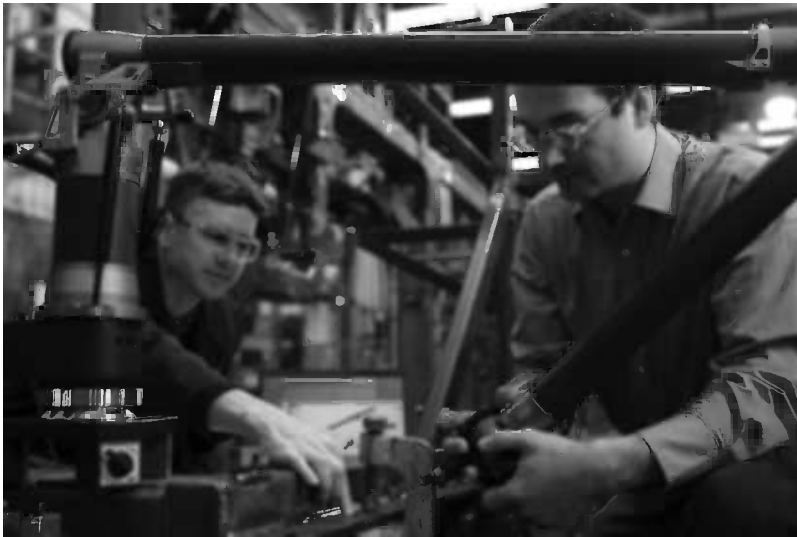
FIGURE 6.9 Example of a rigid measuring setup when using a portable CMM.
