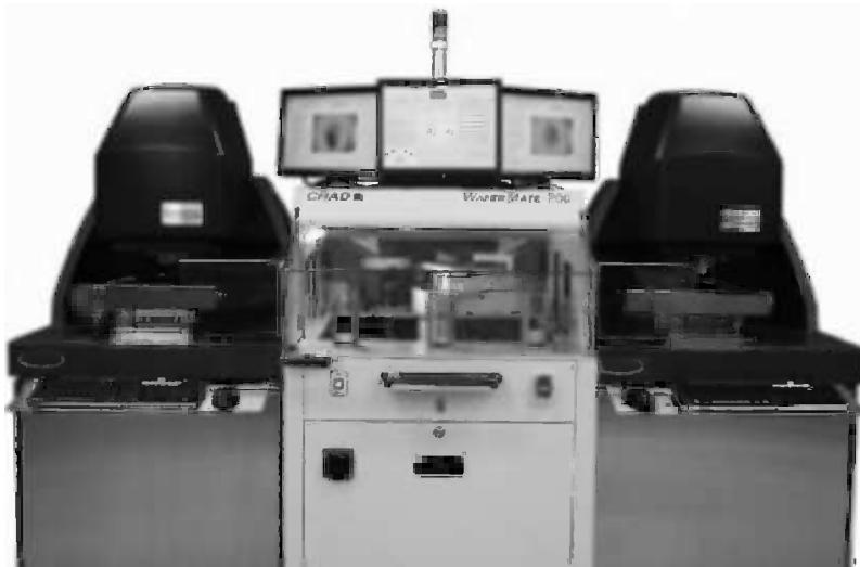
FIGURE 9.14 Two optical profilers sharing a single wafer automation system to help minimize cost.
