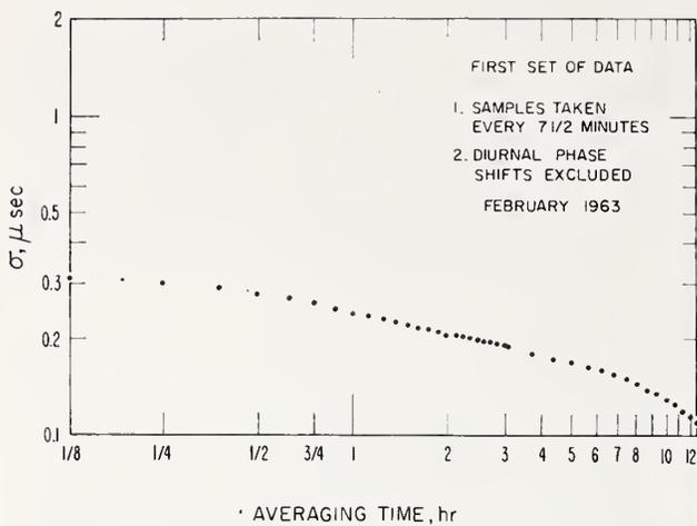
FIGURE 7. *Differential phase stability.*
