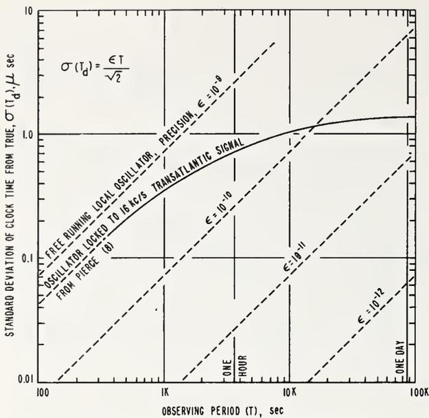
FIGURE 6. Clock-time deviations from original setting as a function of observing period. (<sup>6</sup>Pierce 1957).
