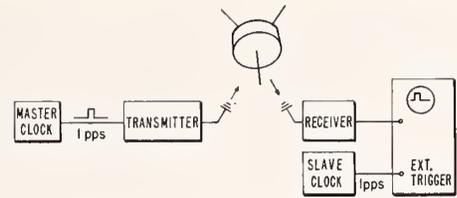
Fig. 1. Block diagram of Mode I clock-synchronization system.
