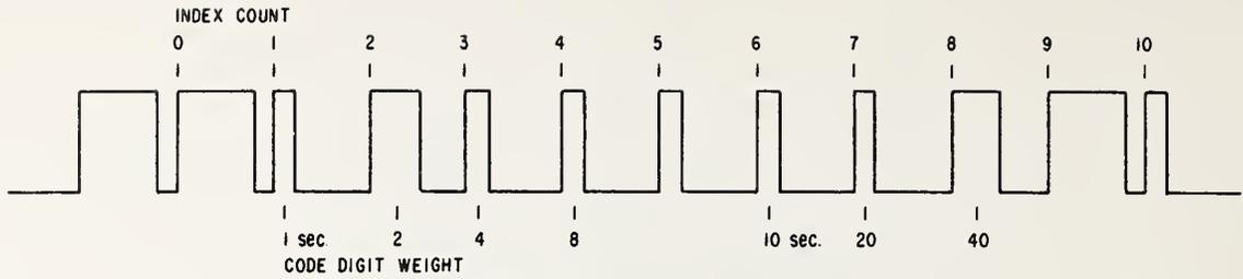
Fig. 9. Example of a 100-pps time code.
