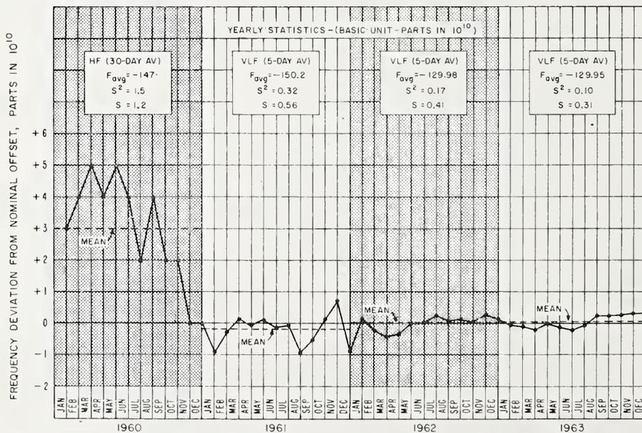
FIGURE 2. Improvements in the frequency control of WWV.
