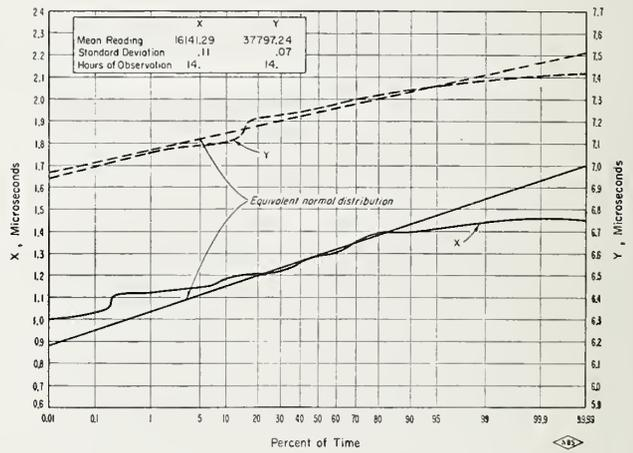
Fig. 14—Cumulative distribution of time difference readings—Kansas (2.5 minute intervals).
