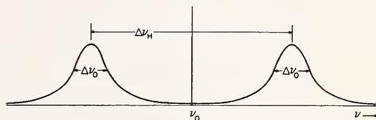
Fig. 1—Zeeman splitting of  $J=3, K=3$  line of N<sup>14</sup>H<sub>3</sub>.
