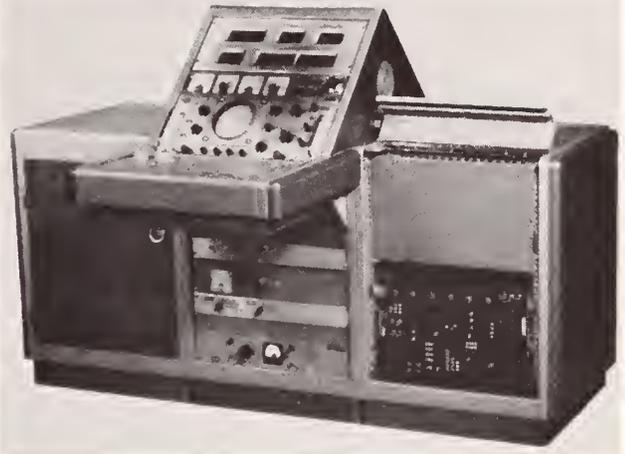
Fig. 4—Loran-C clock.
