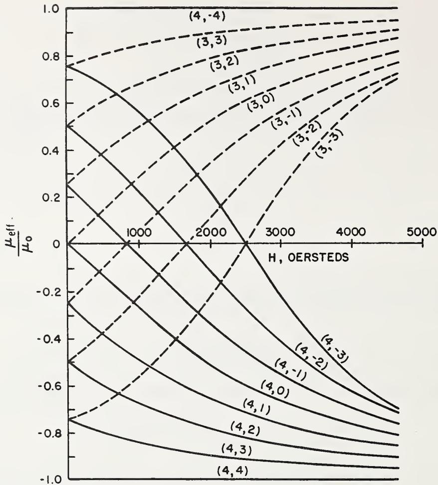
FIG. 9. The effective magnetic moment,  $\mu_{\text{eff}}$ , relative to the Bohr magneton,  $\mu_0$ , is plotted for the various magnetic substates in  $\text{Cs}^{133}$  as a function of the applied magnetic field.
