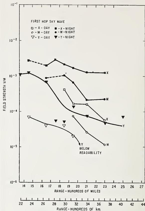
Fig. 35—Field strength of Loran-C sky wave on north-south paths.
