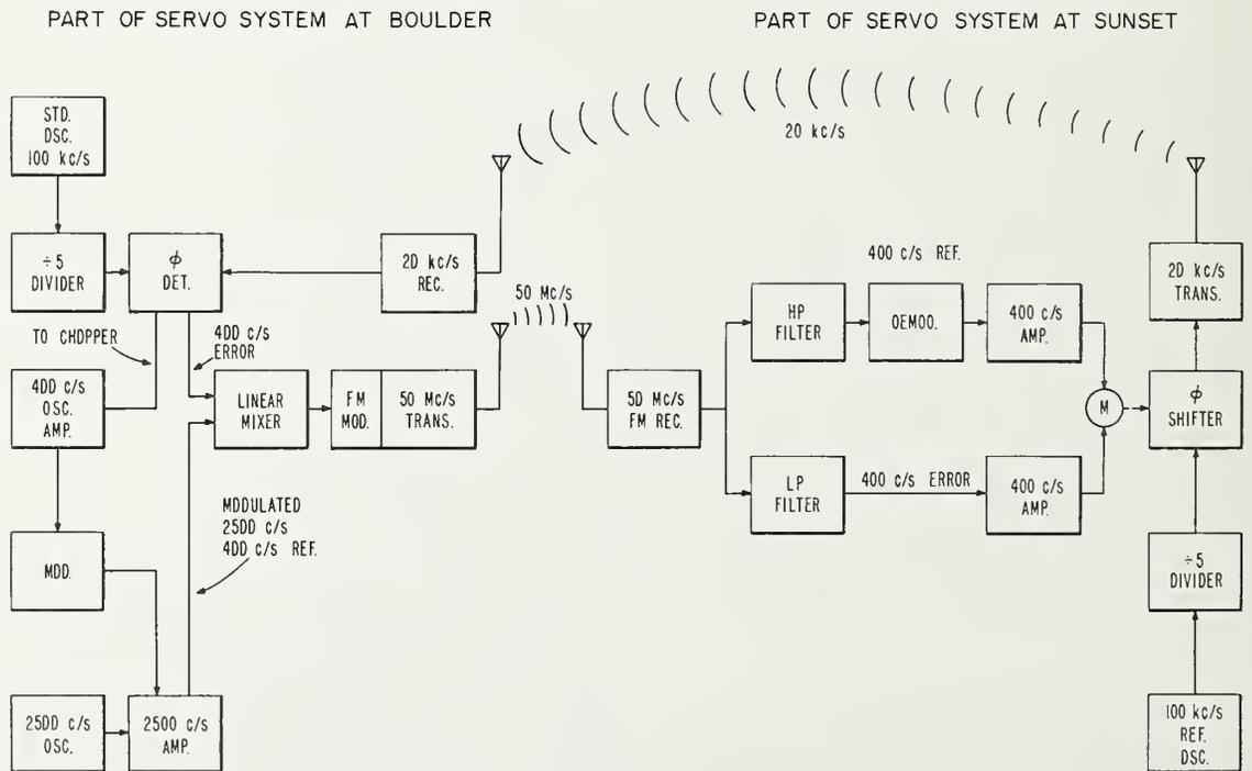
FIGURE 3. Sunset phase-lock system for WWVL (20 kc/s).
