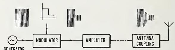
Figure 3. — Simplified block diagram of a transmitter.
