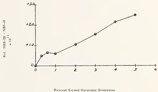
Fig. 8. Relative frequency of NBS III vs. percentage added second harmonic distortion.
