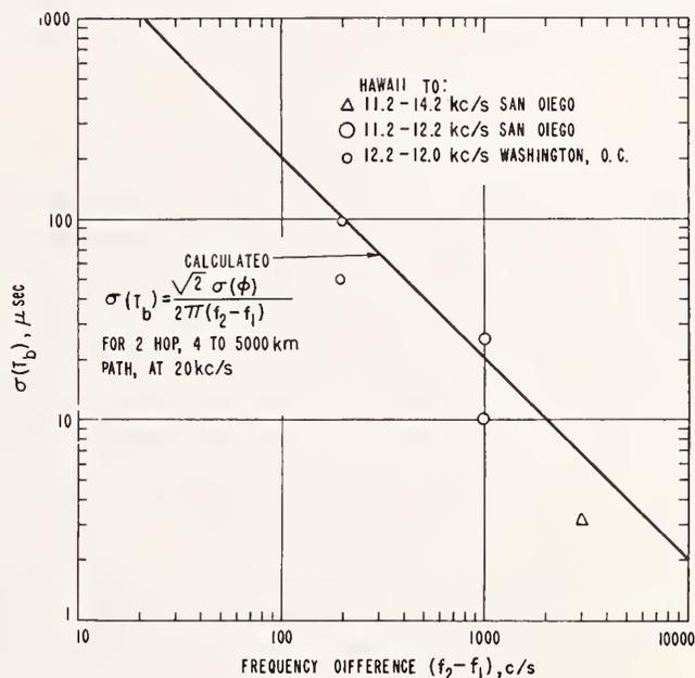
FIGURE 4. VLF transmission path envelope phase stability.
