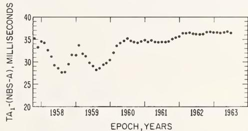
Fig. 9. Comparison of the atomic time scales TA<sub>1</sub> and NBS-A
