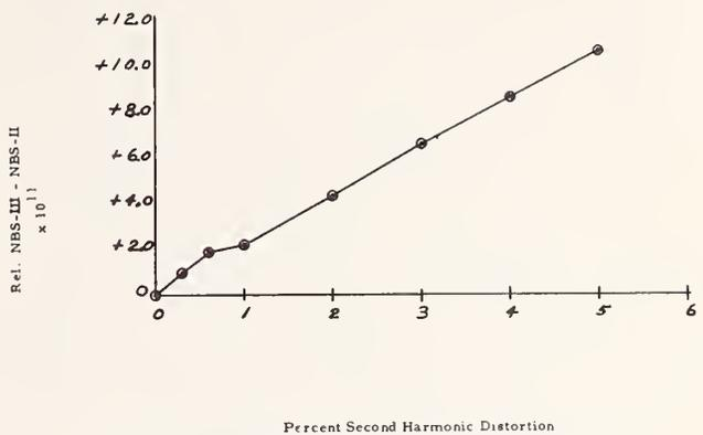
Fig. 7. Relative frequency of NBS II vs. percentage added second harmonic distortion.
