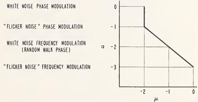
Using (6) and (10) along with the above graph, one may, therefore, deduce the power spectral density from the dependence of the standard deviation of the frequency fluctuations on the sampling time, with restrictions on the experimental parameters as will be shown in the following.
