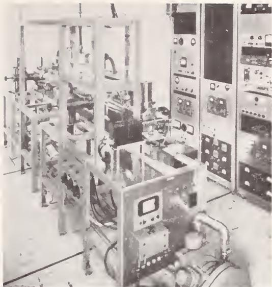
Fig. 1. Cesium atomic beam frequency standard, NBS II.
