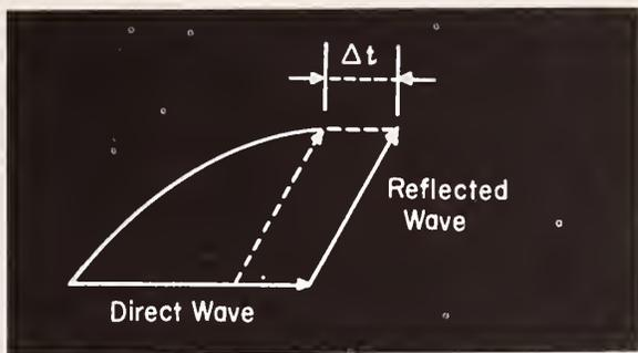
Figure 9. — Vector diagrams for envelope shape.
