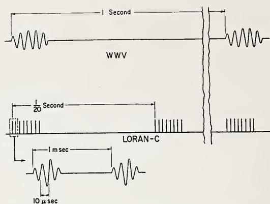
Fig. 3—Synchronization of Loran-C with WWV time signals.
