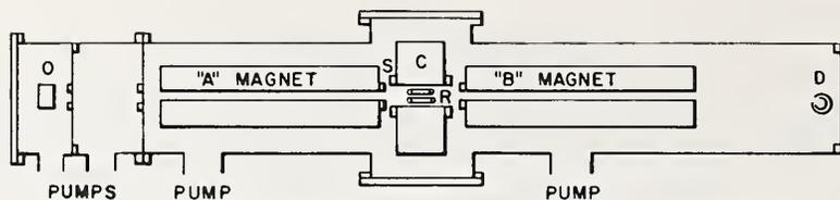
Fig. 2. Schematic diagram of Rabi's magnetic resonance apparatus [5].
