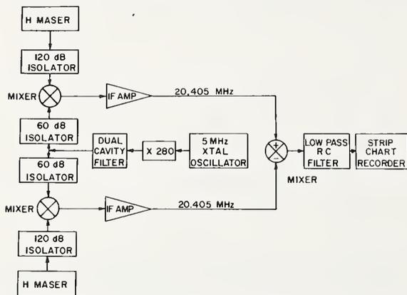
Fig. 14. An alternate system for comparison of *H* masers which avoids the use of phase lock electronics.
