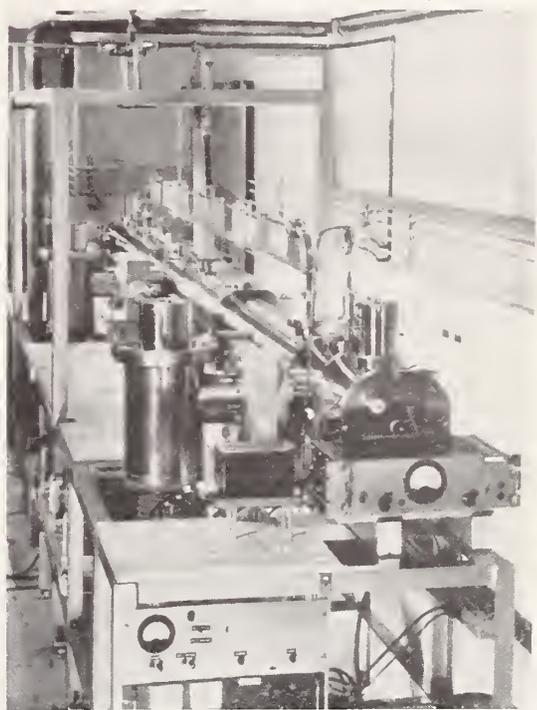
Fig. 2. Cesium atomic beam frequency standard, NBS III.
