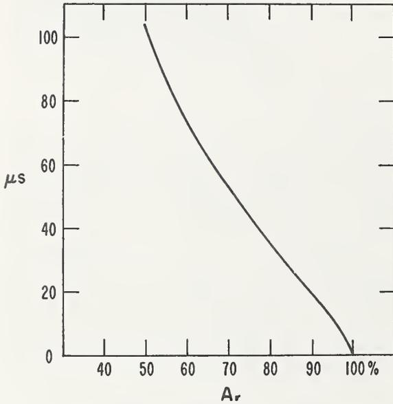
Figure 13. — Timing error due to a 10% variation in "Q" of the transmitting antenna.
