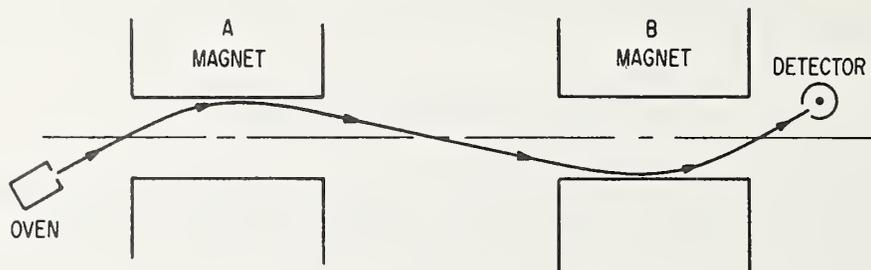
FIG. 12. Oven and detector offset arrangement for the selection of slower atoms. A narrower spectral line results.
