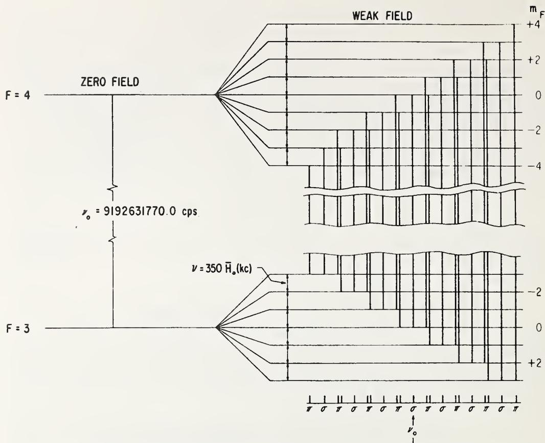
FIG. 5. Energy level diagram for Cs<sup>133</sup>. The nuclear moment is positive,  $I = 7/2$ , and  $J = 1/2$ . The selection rules are  $\Delta F = 0, \pm 1$ ;  $\Delta m_F = 0, \pm 1$ .
