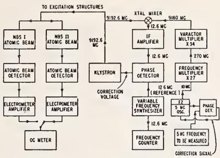
Fig. 1—Block diagram of the manual measurement system.
