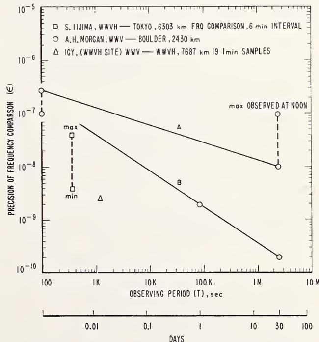
FIGURE 7. Frequency comparison precision at 10 Mc/s.
