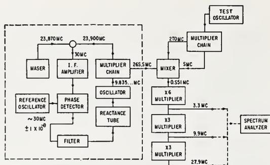
Fig. 9—Block diagram of ammonia-maser-spectrum-analyzer system.
