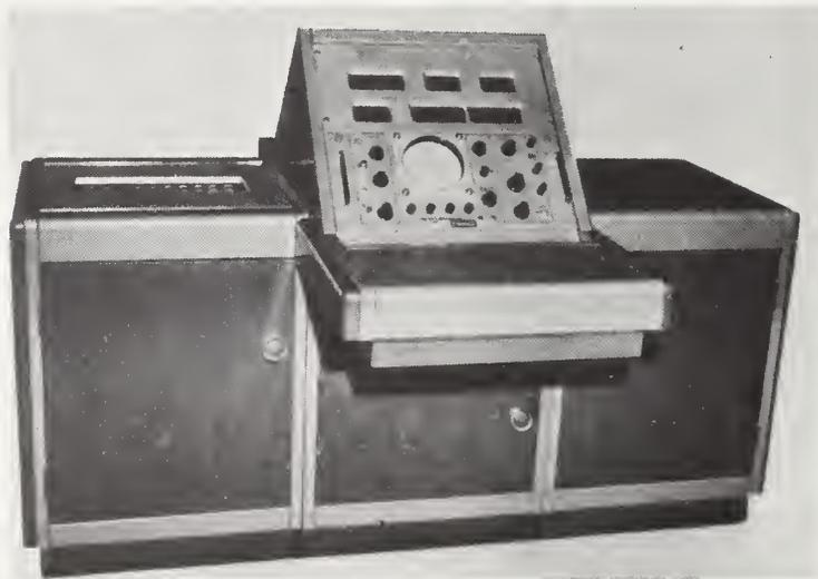
Fig. 2. A Loran-C clock.
