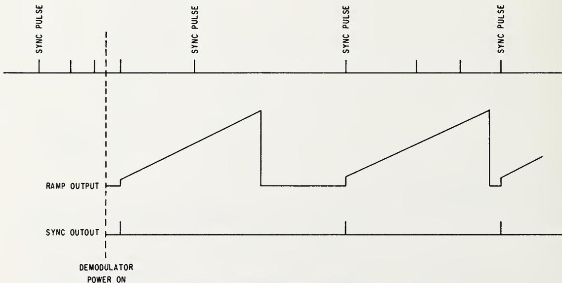
Fig. 14. Demodulator synchronization.
