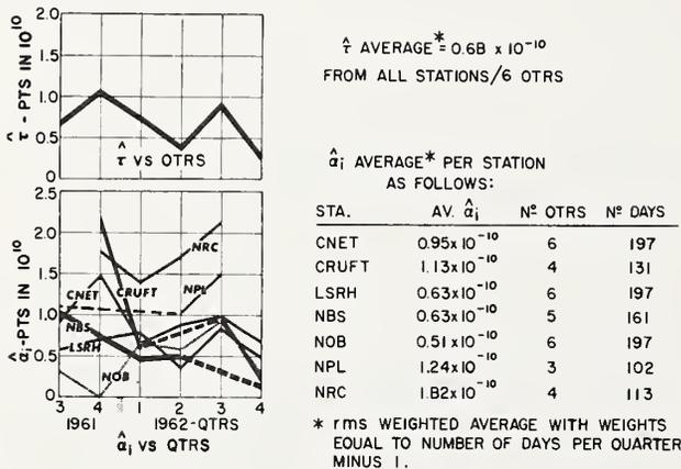
FIGURE 6. Estimated standard deviations,  $\hat{\alpha}_i$ , of receiver variations (including noncommon propagation variations) and estimated standard deviation,  $\hat{\tau}$ , of variations of transmitter NBA (including common propagation variations).
