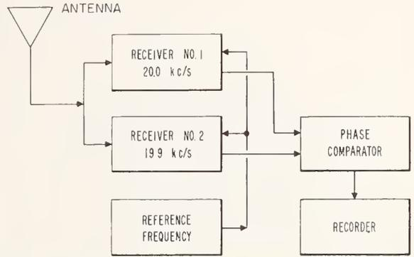
FIGURE 5. Diagram of receiving system at Austin, Tex.
