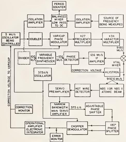
Fig. 2—Block diagram of the servo measurement system.
