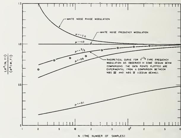
Fig. 1. A plot showing the dependence of the standard deviation of the frequency fluctuation on the number of samples and the type of noise present.
