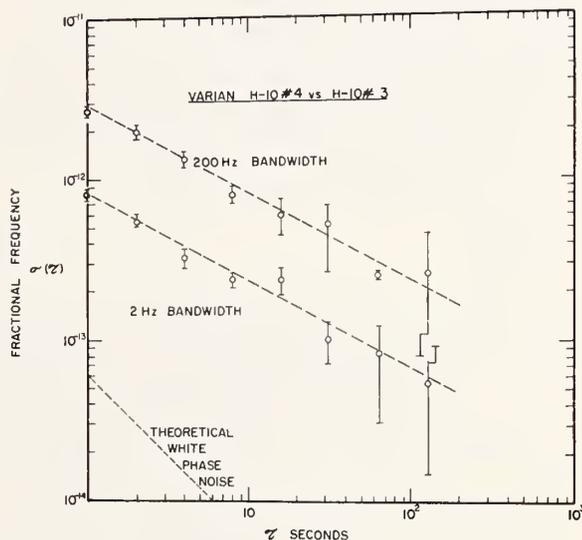
Fig. 11. Standard deviation of fractional frequency fluctuations between *H* masers as a function of sampling time and bandwidth, from automatically printed data.
