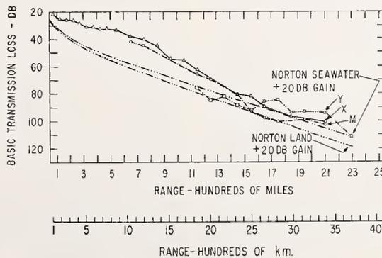
Fig. 29—Predicted and measured ground wave signal amplitude.
