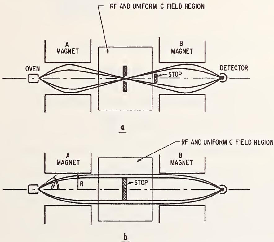
FIG. 15. (a) A beam device designed for  $\frac{1}{4}$  the period of the harmonic motion occurring in the deflection magnet's field. (b) A beam device designed for  $\frac{1}{2}$  the period of the harmonic motion occurring in the deflection magnet's field.
