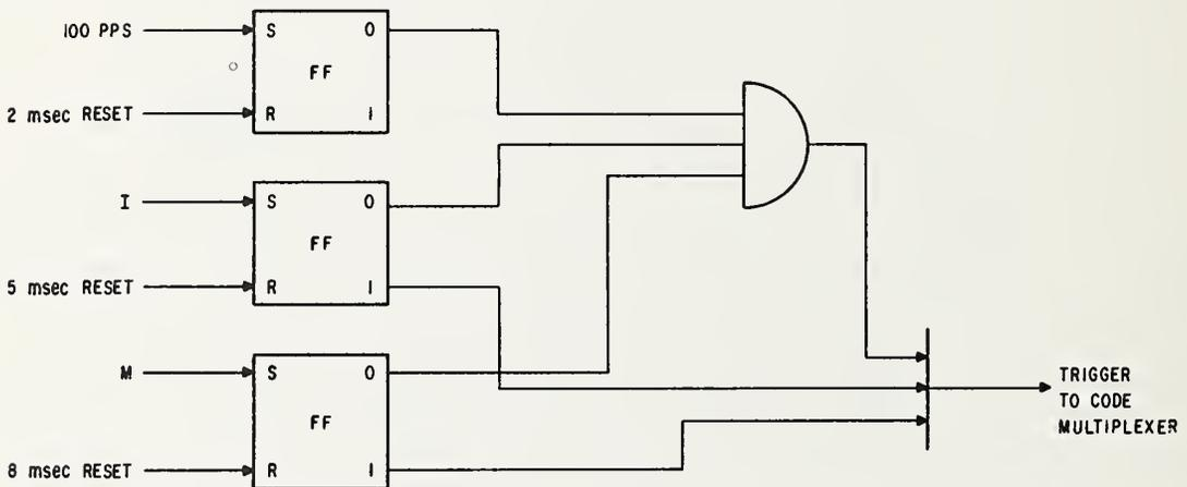
Fig. 10. Example of a 100-pps time code generator.
