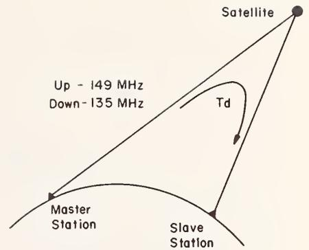
full satellite power levels and the overall system bandwidth is restricted to 100 kHz. For this experiment frequency modulation was employed.
