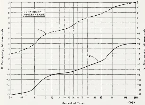
Fig. 10—Cumulative distribution of discrepancy readings—Wisconsin.
