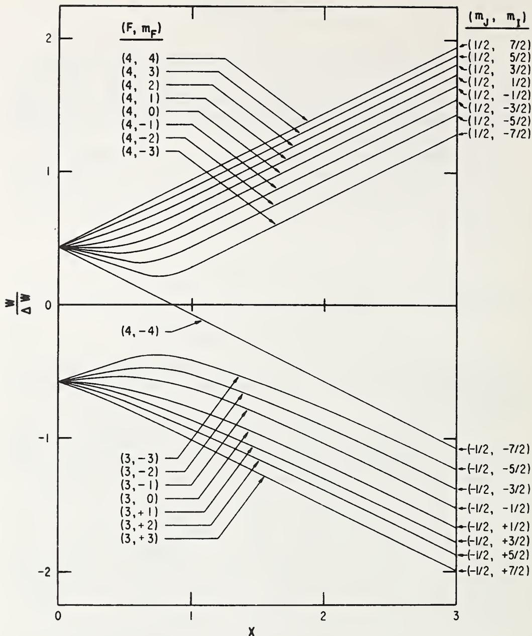
FIG. 7. Energy level diagram of  $\text{Cs}^{133}$  in the  $2S_{1/2}$  ground state as a function of the applied magnetic field. The hfs separation is  $\Delta W = h\nu_0$ .
