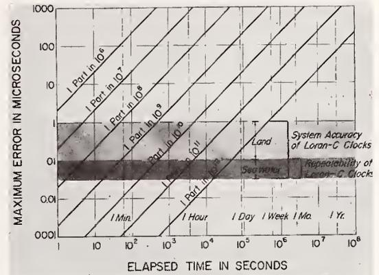
Fig. 5—Comparison of slaved and independent clocks.
