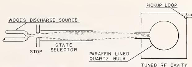
Fig. 15. Schematic diagram of Ramsey's original hydrogen maser [64].
