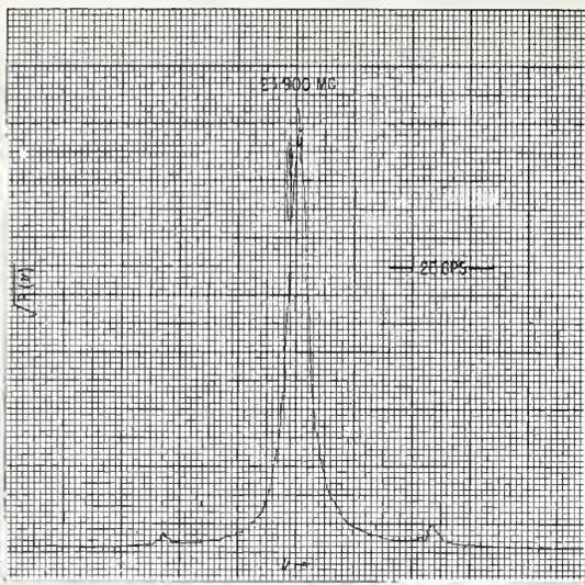
Fig. 3—This spectrum was obtained by intentionally frequency modulating the oscillator of Fig. 2 at a 50-cps rate. The total swing in frequency of the oscillator was about 2 parts in  $10^{10}$  peak to peak. (Note the small sidebands at 50 cps on either side of the central peak.)
