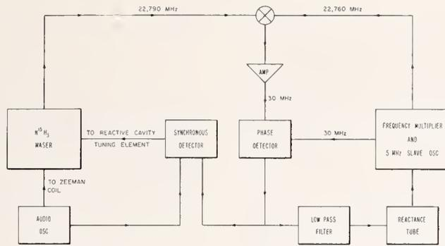
Fig. 3. Block diagram of maser cavity servo system.
