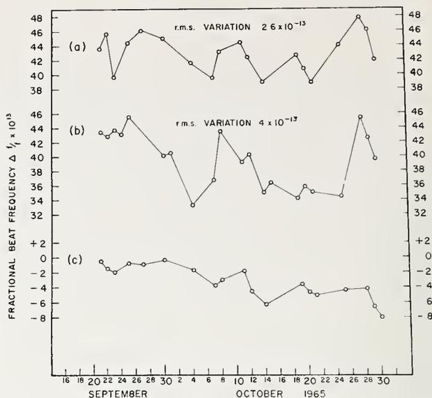
Fig. 16. (a) Fractional frequency difference of *H* masers as a function of time, corrected for cavity tuning effects in both masers. (b) Uncorrected fractional frequency difference of *H* masers as a function of time. (c) Cavity tuning effects in H-10 #4 as a function of time.
