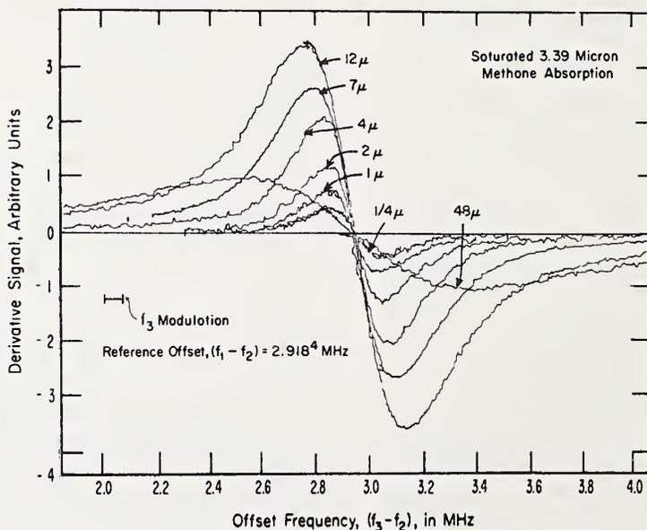
FIG. 2. First derivative of the output power of laser No. 3 versus offset-lock frequency  $f_3 - f_2$ . The several curves are labeled by the  $\text{CH}_4$  (in mTorr) in laser No. 3. Laser No. 1 was stabilized to the center of its methane line. Laser No. 2, local oscillator for both optical-heterodyne detectors, was stabilized against laser No. 1 with a  $2.918^4$ -MHz offset. The curves are very accurately described by the Lorentz-derivative function.
