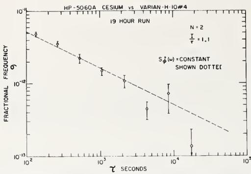
Fig. 7. Standard deviation of fractional frequency fluctuations as a function of sampling time, Hewlett-Packard 5060A vs. Varian H-10 #4; 19 hour run.
