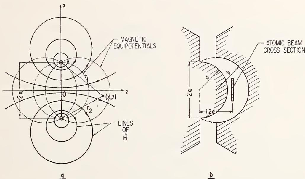
FIG. 13. (a) The field intensity lines and magnetic equipotentials of two parallel wires normal to the diagram at  $x = a, z = 0$  and  $x = -a, z = 0$ . (b) An iron deflecting field contoured to produce a two-wire field.
