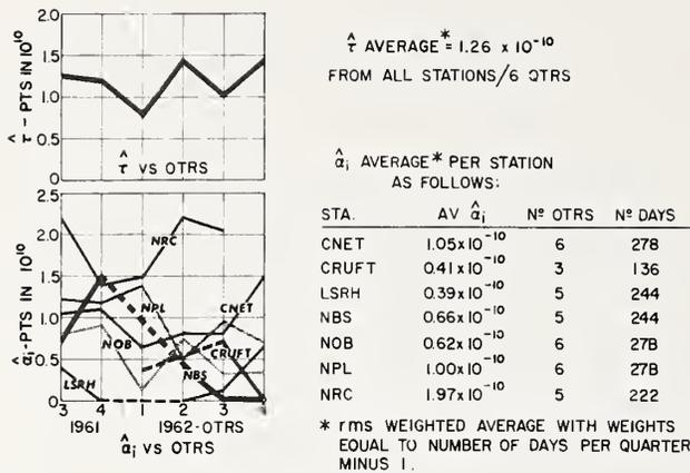
FIGURE 5. Estimated standard deviations,  $\hat{\alpha}_i$ , of receiver variations (including noncommon propagation variations) and estimated standard deviation,  $\hat{\tau}$ , of variations of transmitter GBR (including common propagation variations).
