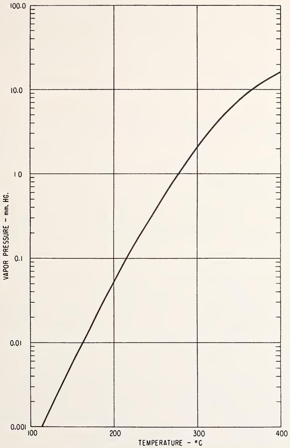
FIG. 18. The vapor pressure of cesium versus temperature.
