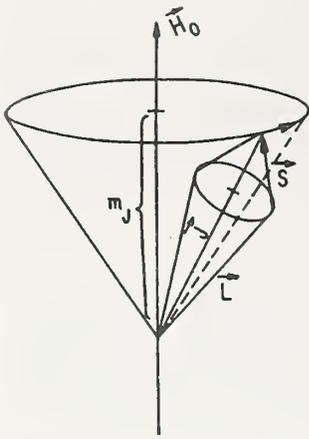
FIG. 4. Vector model of atom with zero nuclear spin.
