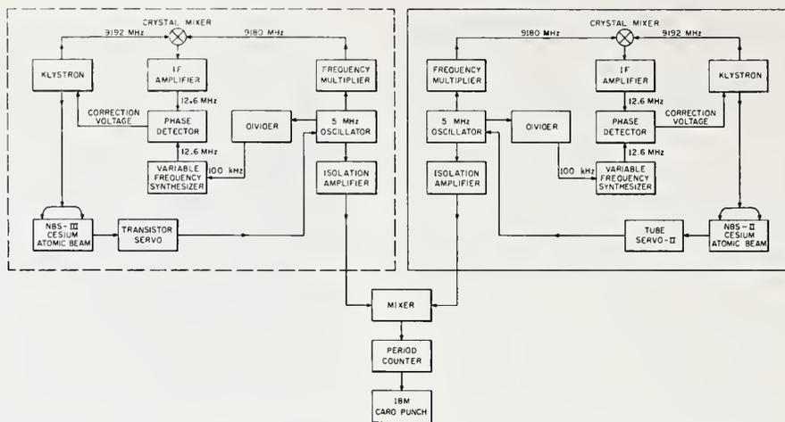
Fig. 3. Block diagram of mixer of measurement system for direct comparison of NBS II and NBS III.
