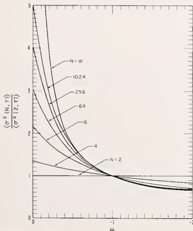
Fig. 2. A plot enabling one to experimentally extract the statistics of an oscillator by knowing the standard deviation for  $N$  samples and for two samples using  $S_{\phi}(\omega) = h|\omega|^{-\mu-1}$  except at  $\mu = -2$ .
