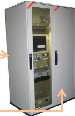
Accuracy 1 fixed calibration system installed in special EMC, temperature controlled racks
