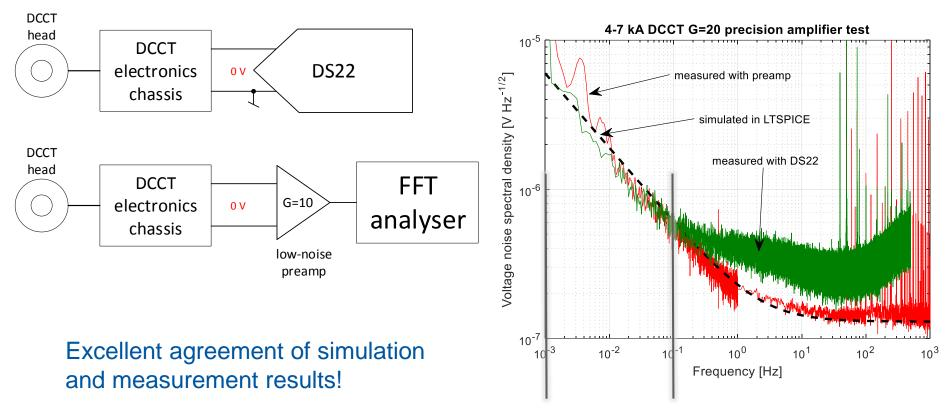
≈330 nV<sub>RMS</sub> from 0.001 to 0.1 Hz Compatible with HL-LHC Class 0
