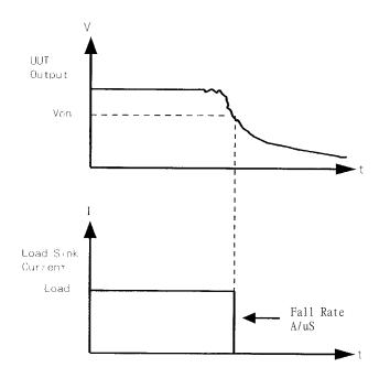
Figure 3-16 Stop Current Loading (Von Non-Latch)
