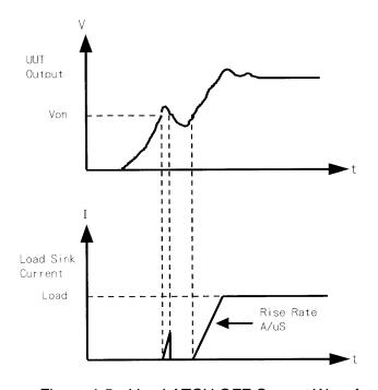
Figure 4-5 Von LATCH OFF Current Waveform
