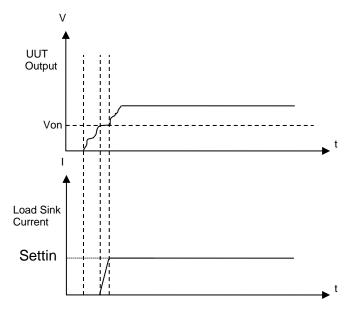
Figure 3-19 When Von Point is set to 0V with Protection
