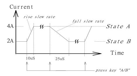
Figure 3-7 Load Level after Pressing **A/B** Key
