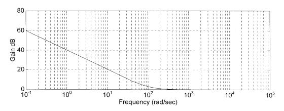
Figure 4-3 CV Response Transfer Function (SLOW)
