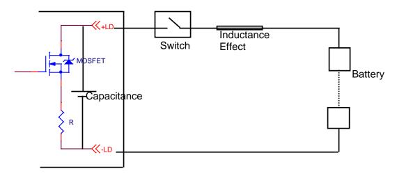
Figure 11-1 Wire Connection of Electronic Load & Battery
