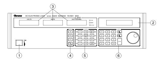
Figure 4-1 Front Panel of the Load
