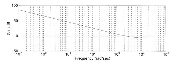
Figure 4-2 CV Response Transfer Function (FAST)
