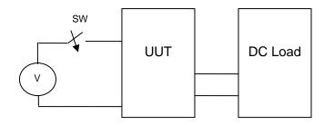
Figure 3-17 Connection of Power, UUT and DC Load
