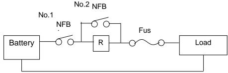
Figure 11-4 Wire Connecting Diagram of LOAD & Battery
