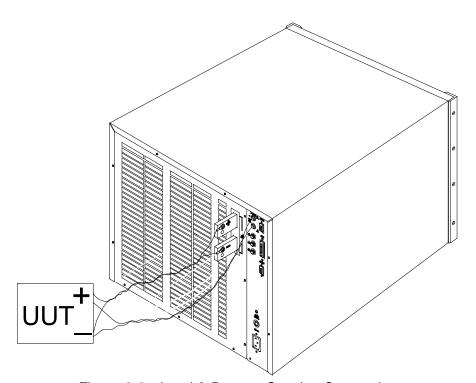
Figure 2-2 Load & Remote Sensing Connection
