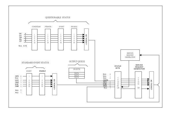
Figure 8-1 The Status Registers of Electronic Load
