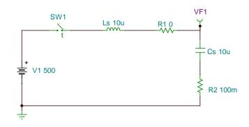
Figure 11-2 Simulated Circuit Diagram
