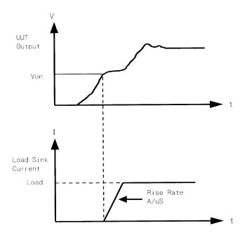
Figure 3-15 Start Current Loading (Von Non-Latch)
