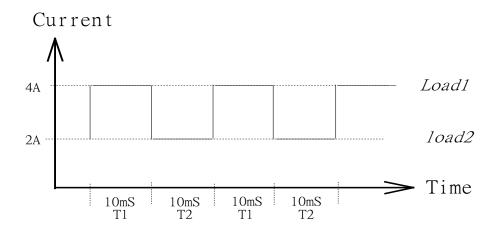
Figure 3-8 Dynamic Current Waveform
