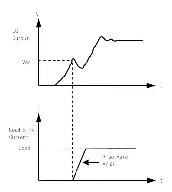
Figure 4-4 Von LATCH ON Current Waveform
