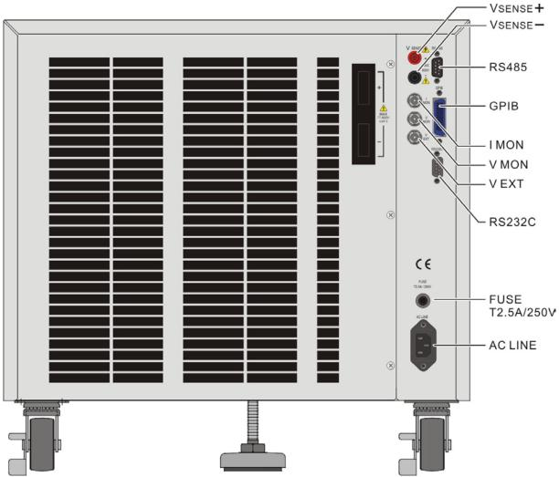
Figure 3-2 Rear Panel of Model 63201/63202/63203/63204
