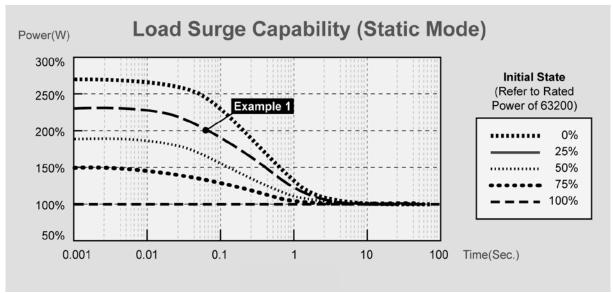
Figure 3-12 Load Surge Capability (Static Mode)
