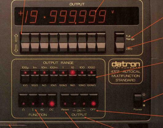
OUTPUT ON APPLIES SELECTED OUTPUT TO TERMINALS. ABOVE 110V (DC) OR 75V(AC), LED FLASHES AND AUDIO WARNING SIGNAL SOUNDS.
