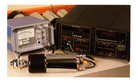
AC Voltage Traceability is provided by the combination of well proven Thermal Converters and 'state of the art' techniques in their use. Such a combination gives the very best performance over a wide range of Voltages and Frequencies.
