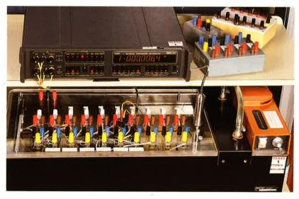
Resistance and AC/DC Current are well provided for by the use of the very best AC/DC Resistance Standards maintained in flowing oil.
