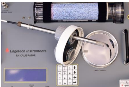
Inserting an RH Probe
