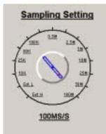
• The knob can be clicked and dragged. When selecting sample between 10KS/S and 100MS/S, system is using internal clock. When selecting Ext L or Ext H, system is using external clock. Ext L is used when external clock is less than 200KHz and Ext H is used when external clock is more than 200KHz.
