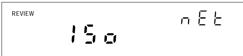
Network display for reviewing the network type (isolated network)
