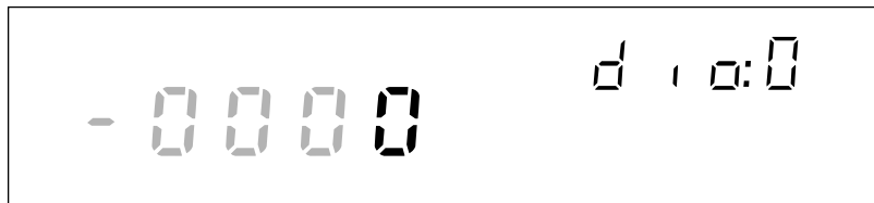
Digital I/O status display for DIO line 0 (for the example 1111-000 0 )
