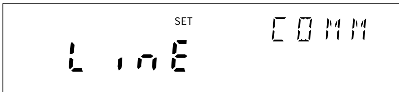
Communications display for setting the line frequency
