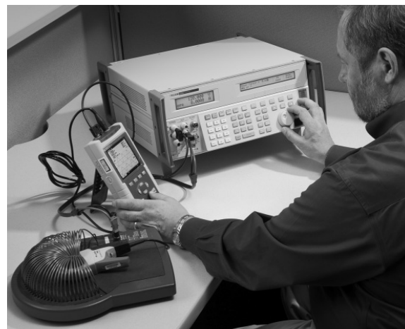
The Fluke Calibration 5522A Multi-Product Calibrator at work calibrating a Fluke power quality analyzer.
