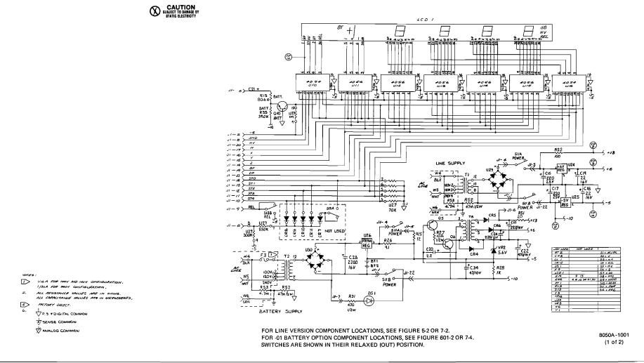
Figure 7-3. A1 Main PCB Assembly, Schematic
