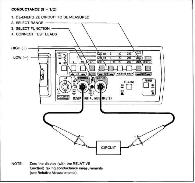
Figure 2-6. Conductance Operation
