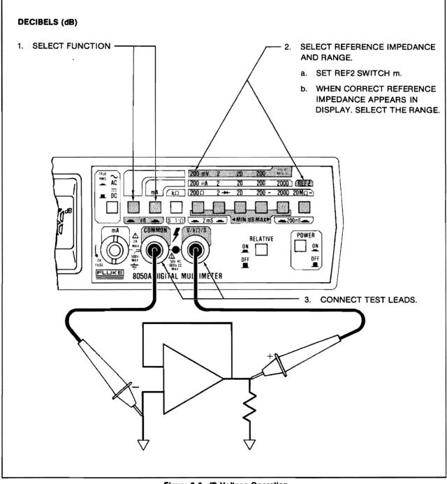
Figure 2-9. dB Voltage Operation
