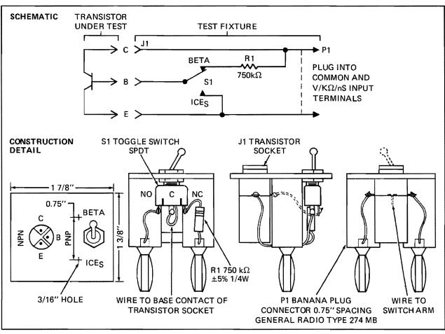
Figure 2-12. Transistor Beta Test Fixture
