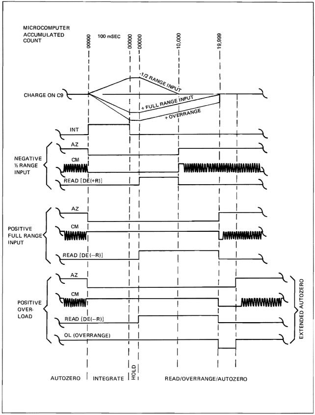
Figure 3-3. A/D Converter Waveforms
