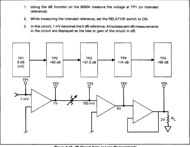
Figure 2-13. dB Circuit Gain or Loss Measurements
