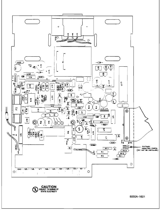
Figure 5-2. 8050A A1 Main PCB Assembly
