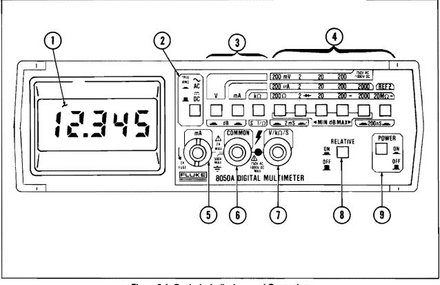
Figure 2-1. Controls, Indicators, and Connectors
