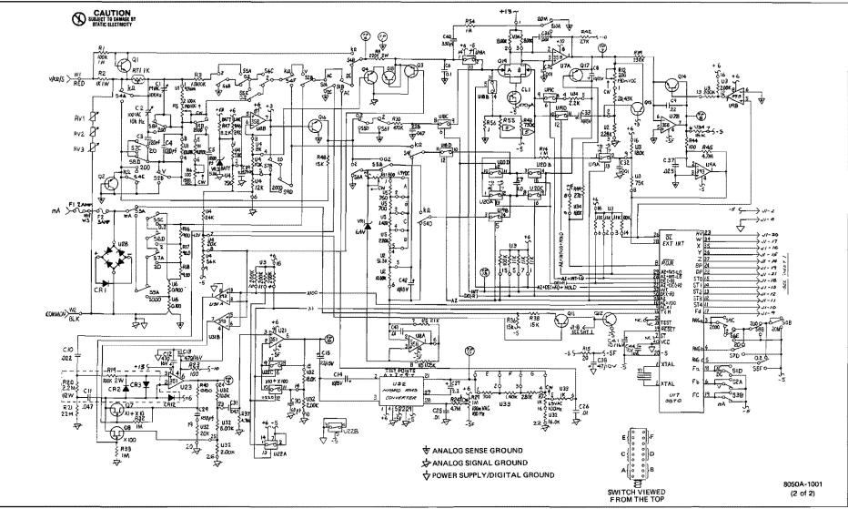
Figure 7-3. A1 Main PCB Assembly, Schematic (cont)
