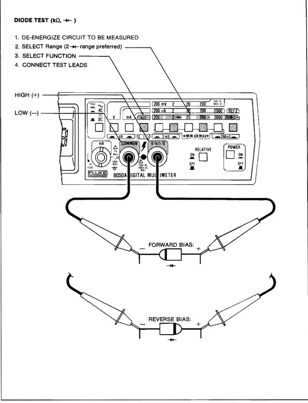
Figure 2-7. Diode Test Operation
