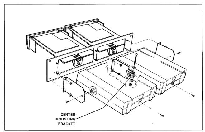
Figure 600-4. Rack Mounting Kit, Side-by-Side Mounting
