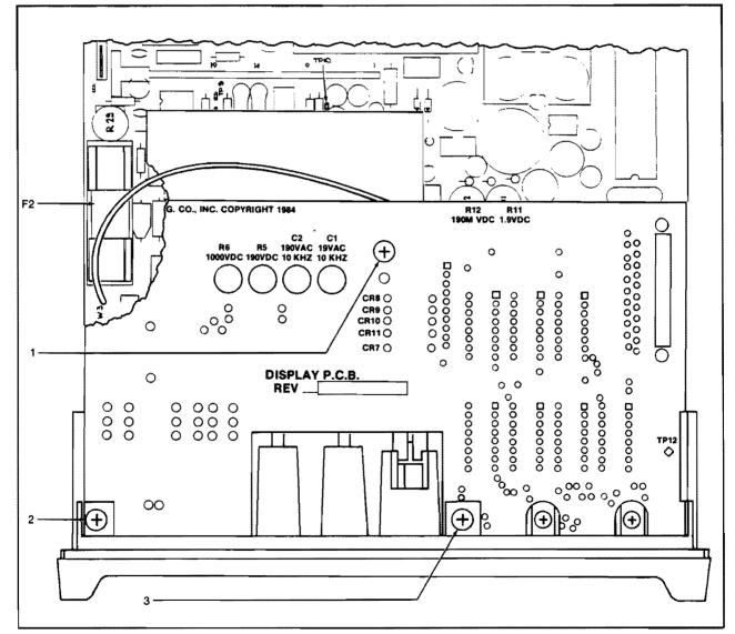
Figure 4-1. Display PCB Access
