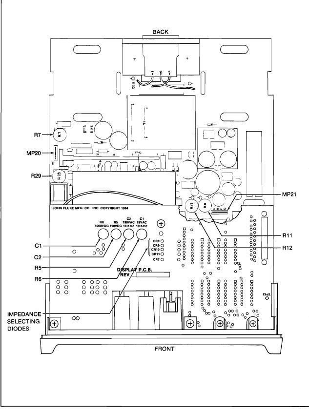
Figure 4-2. Calibration Adjustment Locations
