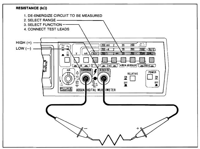
Figure 2-5. Resistance Operation
