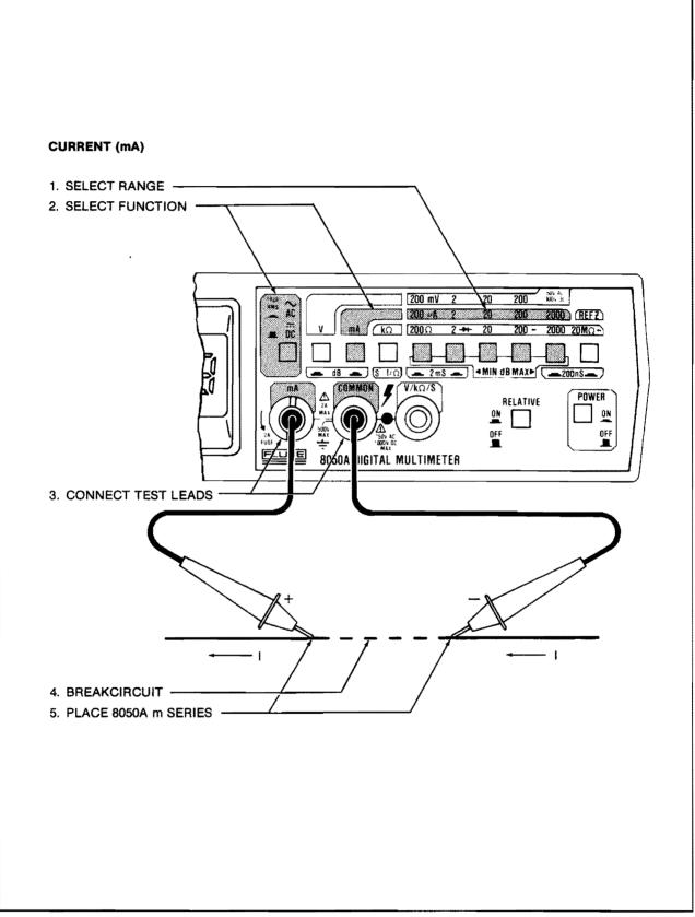
Figure 2-4. AC/DC Current Operation
