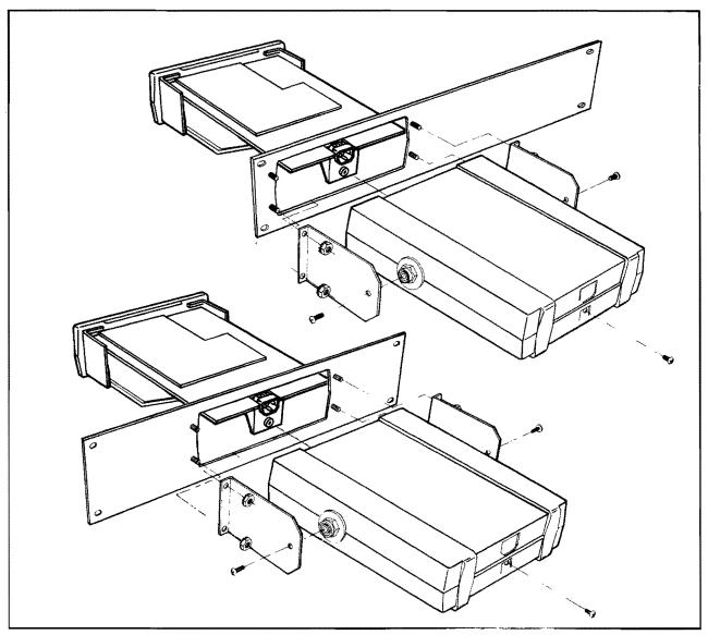
Figure 600-3. Rack Mounting Kits, Offset and Center Mounting
