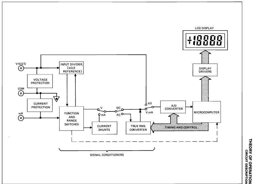
Figure 3-1. 8050A Functional Block Diagram
