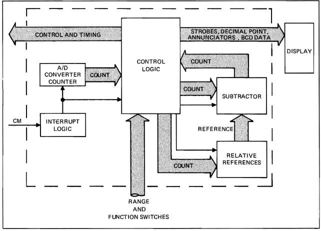
Figure 3-4. Microcomputer Simplified Block Diagram
