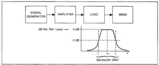
Figure 2-17. Measuring Amplifier Bandwidth
