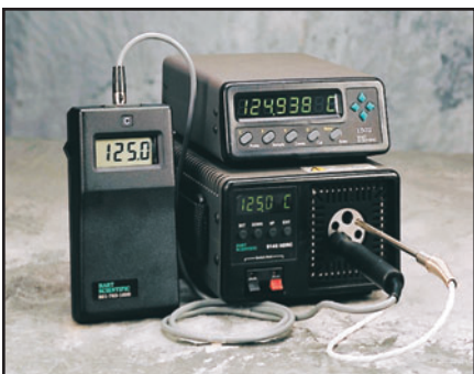
Calibrations using dry-wells can be improved by using an external reference such as the 1502A Tweener Thermometer.
