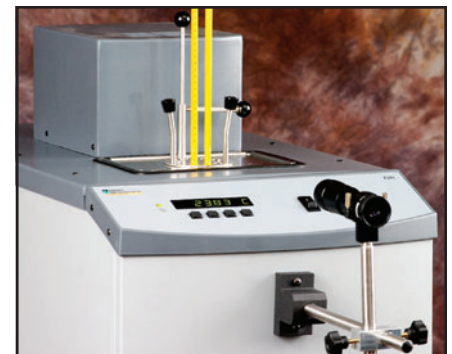
The 2019-DCB Liquid-in-Glass Thermometer Calibration Kit includes a carousel which holds up to 10 thermometers and an adapter tube which raises the bath fluid level to within 5–15 mm of the thermometers' readings. The 2069 Magnifier Scope mounts easily to the front of any Deep-Well Compact Bath to provide magnification of 8X or greater.
