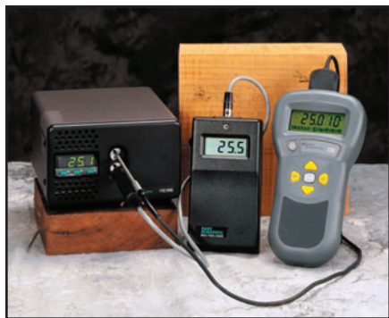
Handheld Thermometers make excellent reference standards for field calibrations.
