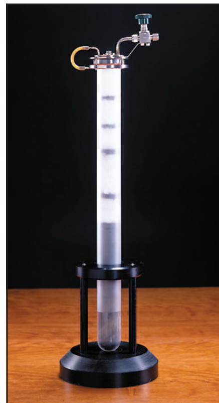
Open cells allow users to minimize the uncertainty from pressure corrections by regulating cell pressures themselves.
