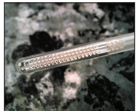
A close-up of a 25-ohm spiral-wound helix SPRT element.
