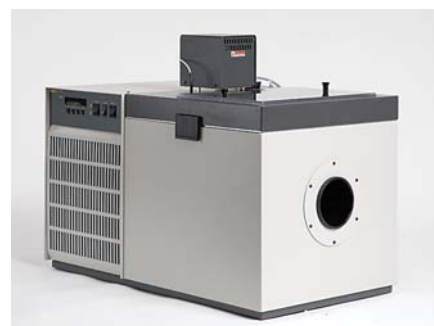
This Hart Model 7008-IR features a NIST-designed cone-shaped target.
