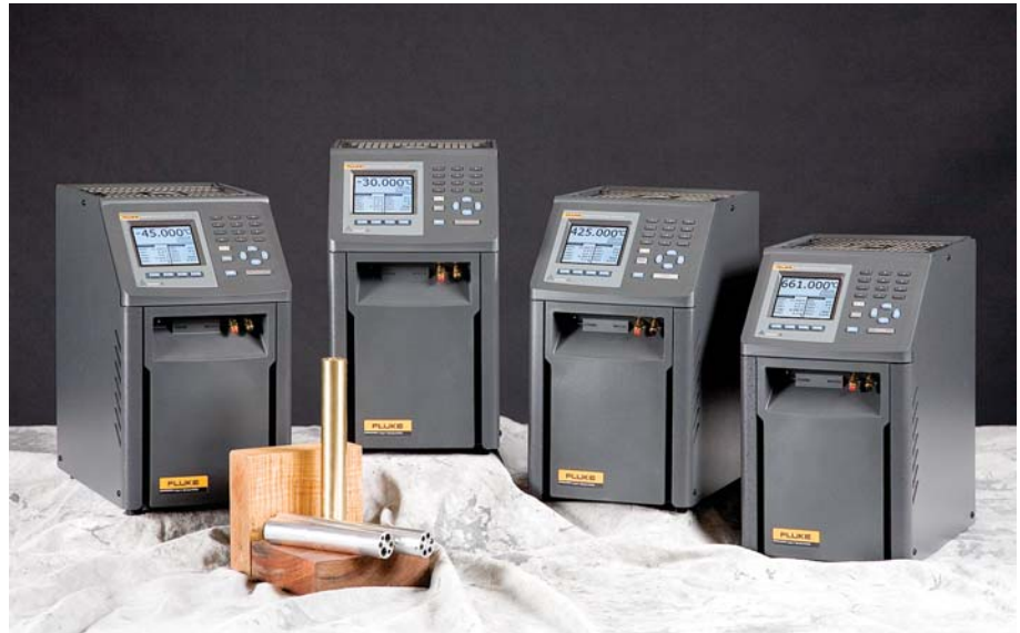
The Metrology Well family consist of four models (Model 9170, 9171, 9172, and 9173) which, combined, cover a temperature range of -45 °C to 700 °C.
