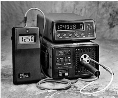
Calibrations using dry-wells can be improved by using an external reference such as the 1502A Tweener Thermometer.
