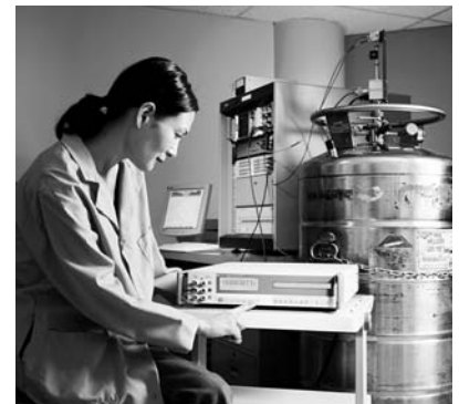
Josephson arrays in US and Germany. Fluke is only one of a handful of commercial organizations operating Josephson Array standards to represent the volt in their metrology operations. Fluke maintains two J-arrays, one at its corporate headquarters in Everett, Washington in the USA, and one in its standards laboratory in Kassel, Germany.
