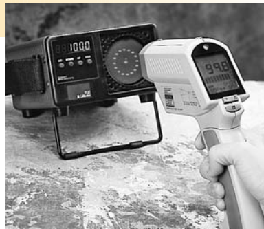
Large target for calibrating all IR thermometer types.
