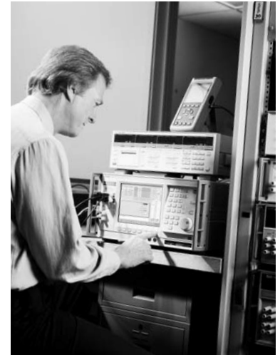
6100 Electrical Power Standard see page 56
