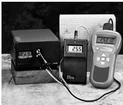
Handheld thermometers make excellent reference standards for field calibrations.
