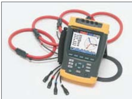
Fluke 435 with flex clamps
