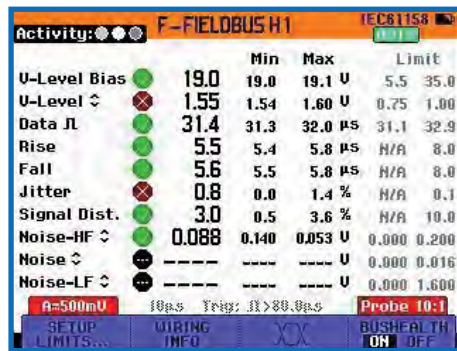
Typical status overview of a bushealth measurement.
