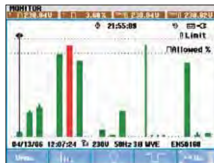
The System-Monitor overview gives instant insight into whether the voltage, harmonics, flicker, frequency and the number of dips and swells fall outside the set limits. A detailed list is given of all events falling outside the set limits.
