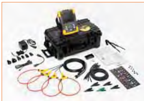
Fluke 437 II with all standard accessories.
