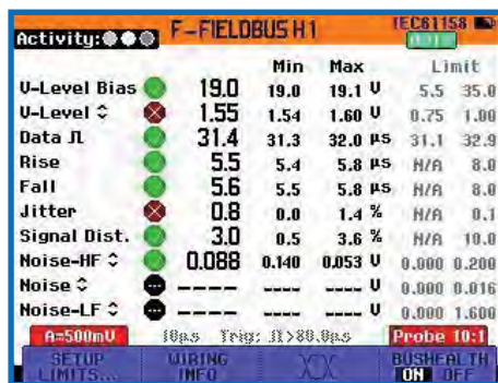
Typical status overview of a bushealth measurement.
