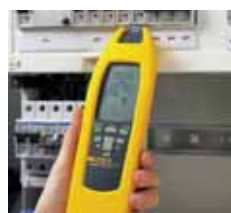
Location of fuses/breakers and assignment to circuits
