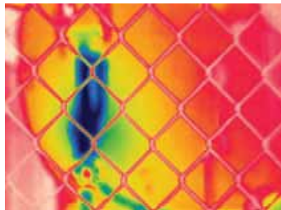
Passive auto focus systems often only capture the near-field subject, in this case the chain link fence
