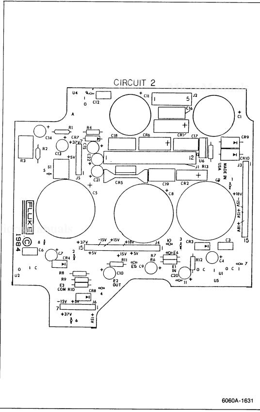
Figure 5-13. A3A1 Power Supply PCA
