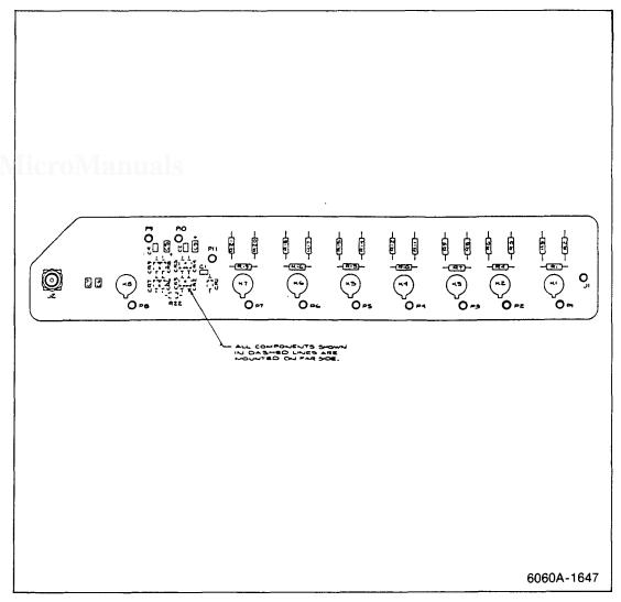
Figure 5-10. A2A5A4 Attenuator/RPP PCA
