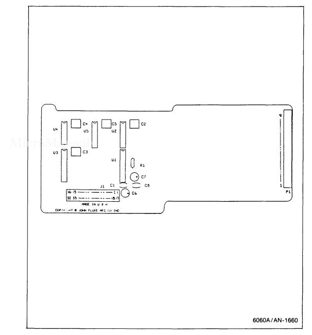
Figure 5-17. A4A2 Analog/Digital PCA
