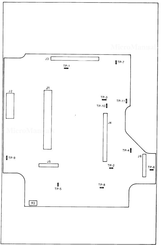
Figure 4C-1. Power Supply Test Points
