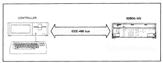
Figure 2-5. 6060A/AN Signal Generator Connected to a 1722A
