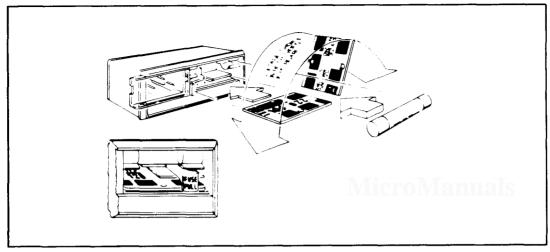
Figure 2-1. Fuse/Filter/Line Voltage Selection Assembly
