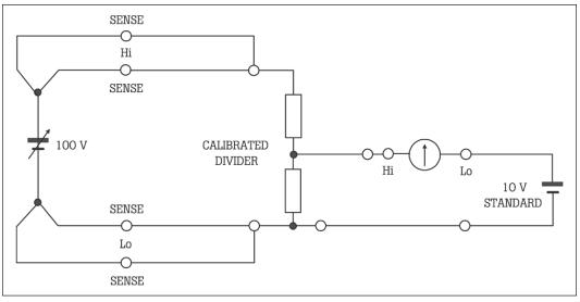
Fig. 6 An example of a Fluke 7105A or datron 4900 voltage calibration system
