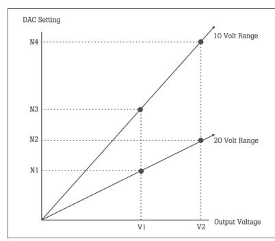
Fig. 5 Converter linearity verification
