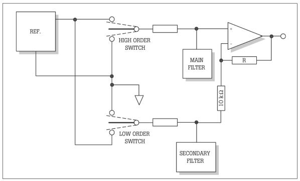
Fig. 3 Two stage PWM circuit
