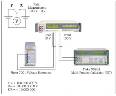
**Fig. 7** An example of the reference multimeter being used to accurately verify the output of the artifact calibrator to a known voltage reference
