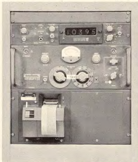
500-Mc frequency meter, with printer. Includes Type 1143-A Frequency-Measuring Assembly and Type 1137-A Data Printer.
