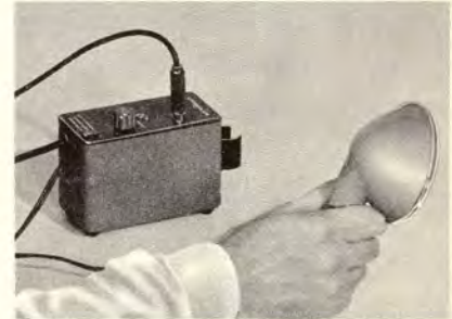
Lamp, at end of five-foot cable, can be held in hand as shown here or attached to case as shown below, left.
