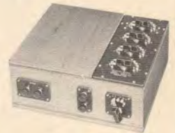
Type 216 Capacity Bridge 1920
