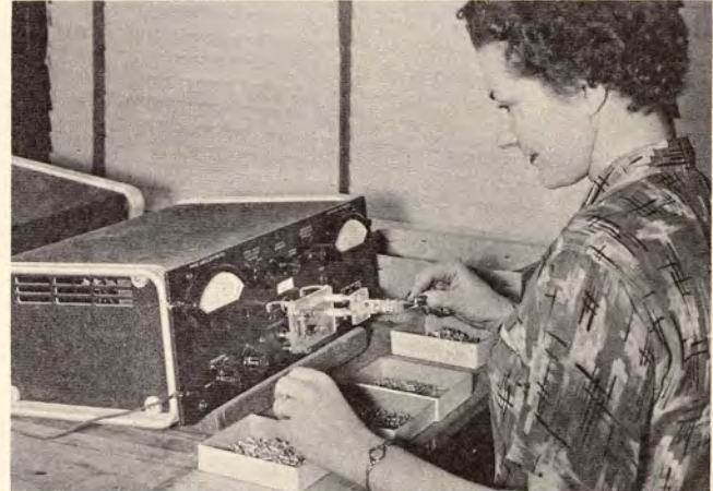
The GR Impedance Comparator in use for production testing of capacitors at Centralab's Milwaukee plant.
