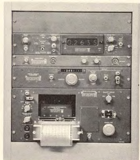
100-Mc recording frequency meter. Includes Type 1144-A 100-Mc Digital Frequency Meter and Discriminator and Type 1510-A Digital-to-Graphic Recording Assembly.
