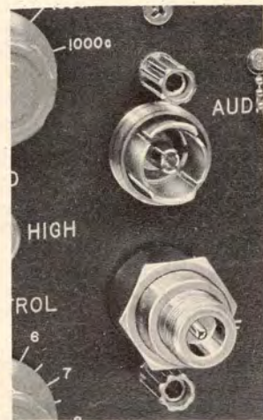
locking GR874 panel connector converted to type N with Type 874-QNJL Adaptor
