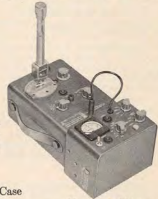
The Type 1556-B Impact-Noise Analyzer attaches to the Type 1551-C Sound-Level Meter as shown here.
