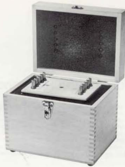
1444-A 10-k \Omega standard with temperature sensor, shown with carrying case.
