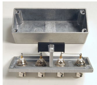
The 1 MΩ resistor is used to check the upper ranges of various LCR meters. The metal bracket serves as both support and shield.
