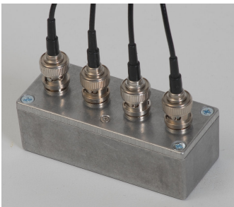
The 1 MΩ resistor is used to check the upper ranges of various LCR meters. The metal bracket serves as both support and shield.
