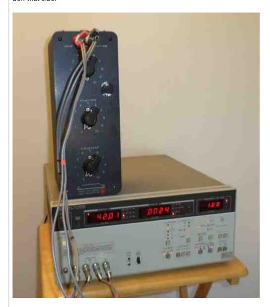
And how about it's non-zero value accuracy? Below all the switches are set to "10" so the total capacitance should be 1.110 uF.
