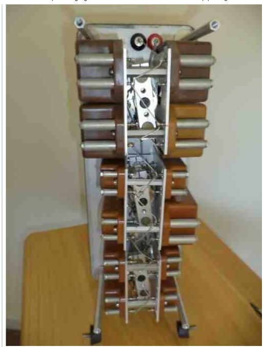
And here is a closeup of some of the standard capacitors, "type 980". The smaller one on the right is the only cap in the box that doesn't have a printed (or stamped?) label... it appears to be labeled by hand. I wonder why?
