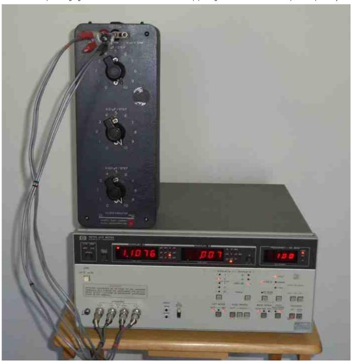
Note that the measured value, 1.1076 uF, only differs from the spec sheet by 0.2% (OK, the error is really in combination with the HP 4276A's accuracy, which is about 0.1%). This result is well within the 1419-K's original spec of 0.5%!
