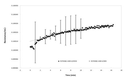
stability of a Guildline 6623A-PCS. With this Guildline designed DC Current Transformer, current Stabilities as low as 5 ppm were measured. The upward drift noted in the chart is the self-heating effects of the shunts.
