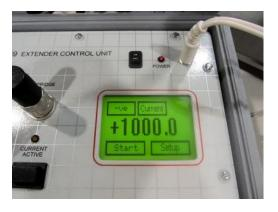
and associated wiring. This completely self-contained precision current source allows you to fully automate calibration procedures.
