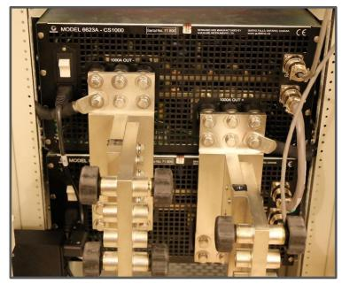
Ampere increments. Of course, with the modularity provided by the patented PCB boards, any customer specified value in 150 Ampere increments from 150 Amperes to 10,000 amperes can be provided. For example, 1200A, 2550A, 3300A, etc. are available outputs as is any value that is in 150 Ampere increments starting from 150A.
