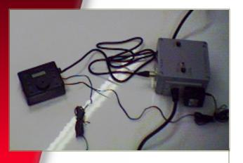
G uildline 50103 Over-Under Temperature Protector serves to protect fixed-temperature or programmable-temperature fluid baths from straying out of a pre-defined temperature range due to a malfunction of the bath temperature control.
