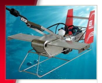
he Guildline 8820A MiniBAT is an extremely lightweight, remotely controlled towed instrumentation platform designed for use with a wide variety of data collection instruments. It provides a highly flexible profiling system for use in estuaries, lakes, rivers, and coastal areas. Deployment of the MiniBAT is made simple by the provision of the easy-to-use Windows based software and by a control box for automated or manual operations. The control box also provides an emergency override capability.
