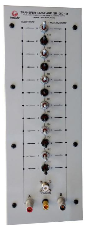
resistance elements can be realized. Based on a unique method for establishing known ratios, the Model SR1050 standard utilizes a transfer technique that consists of switching resistance sections in parallel, series or series-parallel sections.
