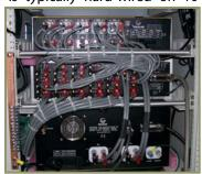
When installed, the DMM Switch allows the 6625 operator to use the System either in a measurement configuration against the 6622 Series Bridge or allows the 6634A resistance values to be used as a Standard output on any available free scanner channel without having to change wires or remove cables.
