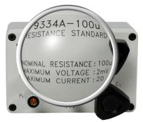
no more than 15 ppm from initial calibration value. Then for the 2<sup>nd</sup> year of use, the unit should not drift any more than 10 ppm and will get better with time.
