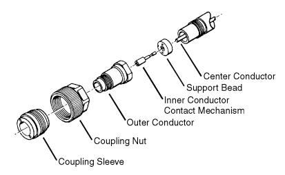
Figure 9 APC-7 Connector Parts Diagram
