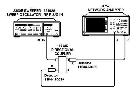
Figure 8 Test Equipment Setup for Agilent 11692D
