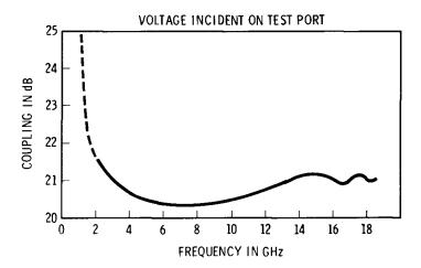
Figure 2 Voltage Incident on Test Port
