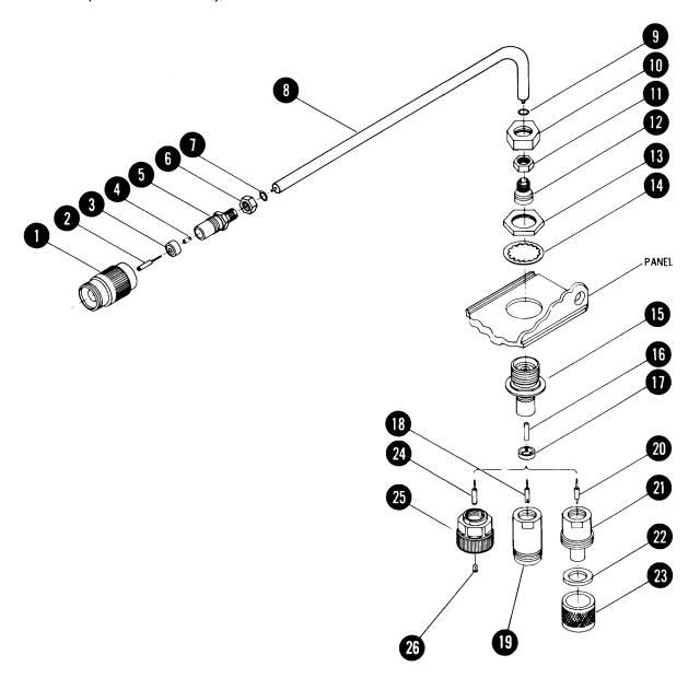
Figure 11 Agilent 11691D Coaxial Line Removal/Replacement
