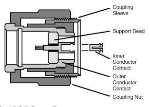
Figure 10 Replacing the APC-7 Center Contact
