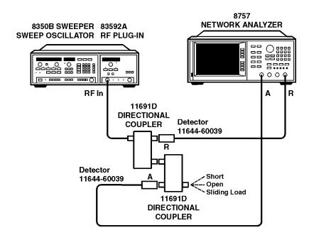
Figure 7 Test Equipment Setup for Agilent 11691D
