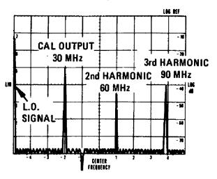
Figure 4-1. 30 MHz Calibrator Signal and Harmonics
