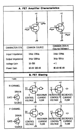
Figure 8-8. Field Effect Transistor Operation.
