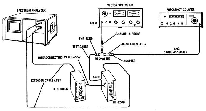
Figure 5-6. 150 MHz Oscillator Adjustment Test Setup
