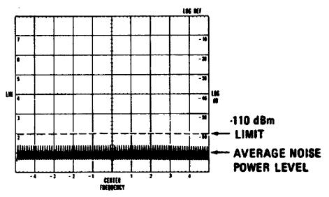
Figure 7-1. Sensitivity Measurement: CRT Display.
