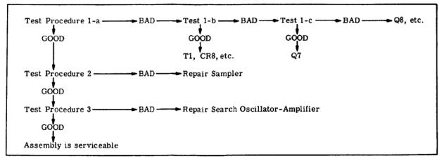
Simplified Test Procedure Tree
