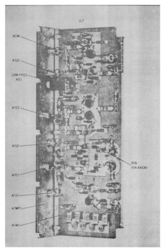
Figure 8-32. 200 - 310 MHz VTO Assembly A7 (08553-6003) Component Locations (CHANGE 8)
