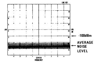
*Figure 7-3. Residual Response Test:* 10 to 110 MHz CRT-Display.
