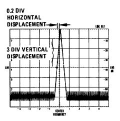
Figure 4-15. Demodulation Sensitivity Measurement.
