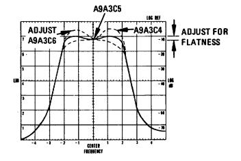
Figure 5-5. 200 MHz Bandpass Shape Adjustment: CRT Display
