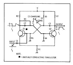
Figure 8-7. Basic One-Shot Multivibrator Circuits.
