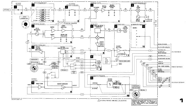
Figure 8-19. Block Diagram of 8553B RF Section
