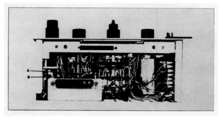
Figure 8-49. Bandwidth Switch A1 (08553-60126) Test Points
