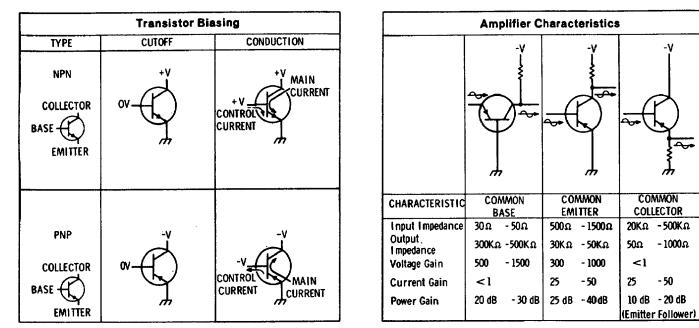
Figure 8-3. Transistor Operation.
