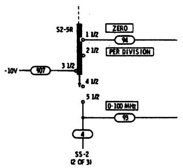
P/O Figure 8-48. Bandwidth Control Circuits for IF Section (ERRATA)
