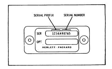
Figure 1-2. Instrument Identification
