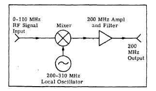
Figure 8-27. Functional Block Diagram.
