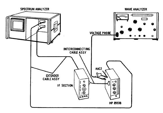
Figure 5-14. APC 100 kHz Rejection Adjustment Test Setup
