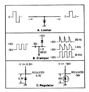
Figure 8-9. Basic Diode Circuits.
