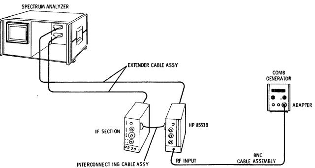
Figure 5-15. APC Tuning Stabilizer Final Check Test Setup
