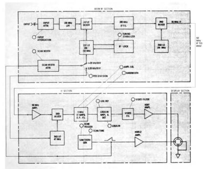
Simplified Analyzer Block Diagram
