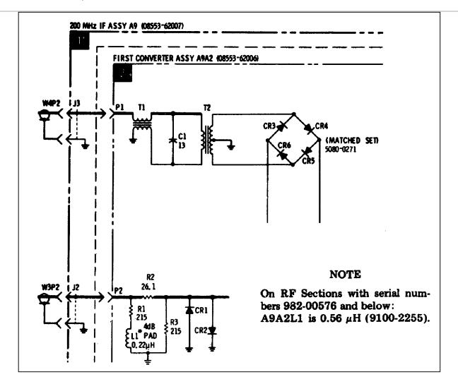
Figure 7-4. H01/H02 Schematic Changes for Service Sheet 4, Figure 8-31.
