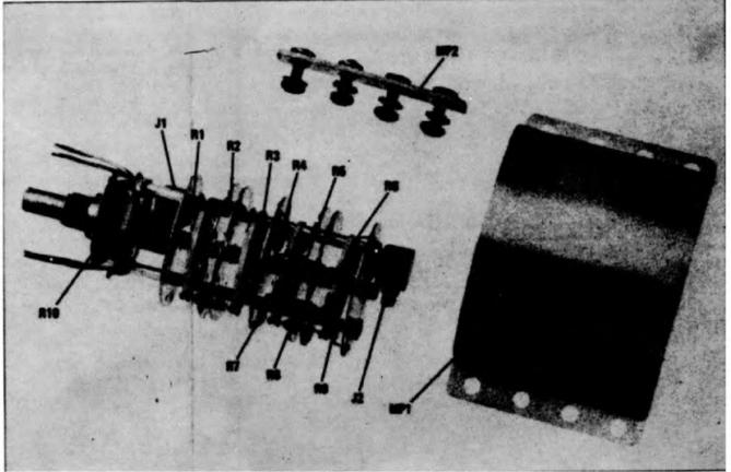
Figure 8-22. Input Attenuation Assembly A3 (08553-6021)
