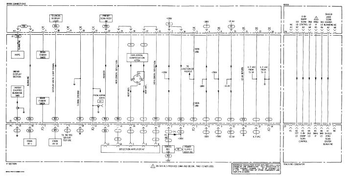
Figure 8-51. RF Section, Display Section Interconnections
