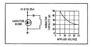
Figure 8-12. Varactor Characteristics.
