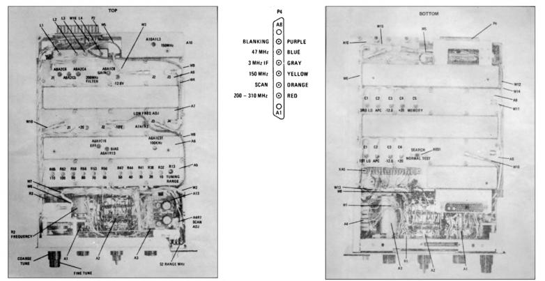
Figure 8-18. 8553B Assembly and Adjustment Locations (Top and Bottom View)
