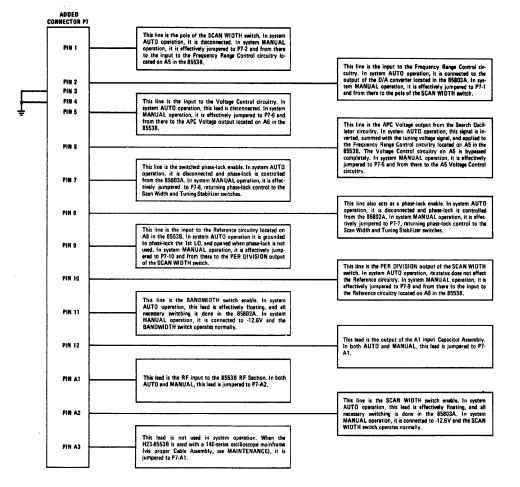
Figure 1. Connections to Added Connector P7
