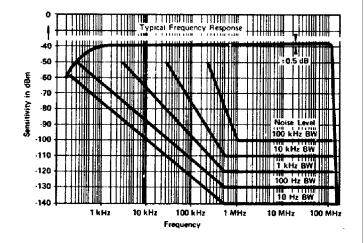
Figure 1-4. Typical Frequency Response
