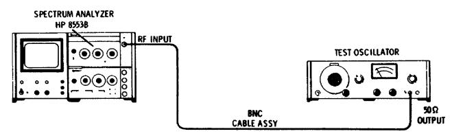
Figure 4-10. Frequency Response Test: 1 kHz to 10 MHz
