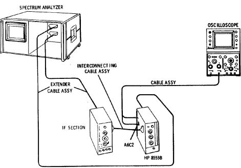
Figure 5-13. APC Search Oscillator Check Test Setup.
