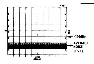
Figure 4-11. Sensitivity Measurement: CRT Display
