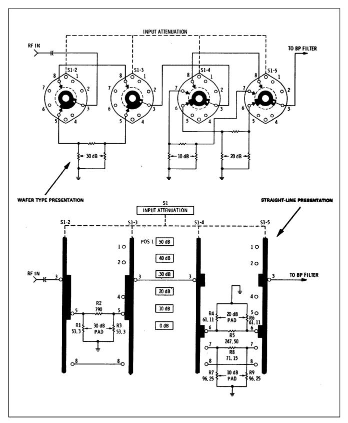
Figure 8-16. Wafer Switch Presentation Versus Straight-Line Presentation
