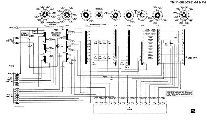
Figure 3. Overall Wiring and Switching Diagram (replacement for Service Sheet 2(3 of 3) in 8553B Operating and Service Manual)
