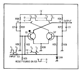
Figure 8-6. Basic Flip-Flop Circuits.
