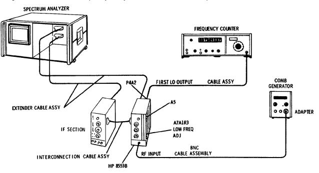
Figure 5-1. First Local Oscillator Adjustment Test Setup
