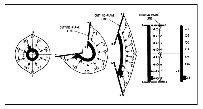
Figure 8-14. Evolution of Straight-Line Switch Presentation
