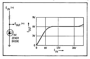
Figure 8-11. Zener Diode Characteristics.
