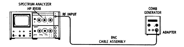
Figure 4-5. Scan Width Accuracy Test: 10 MHz/Div
