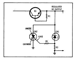
Figure 8-10. Silicon Controlled Rectifier used as a Crowbar.
