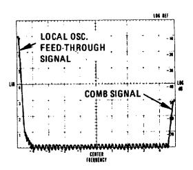
Figure 5-2. First Local Oscillator Adjustment: CRT Display
