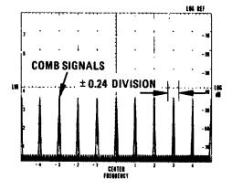
Figure 4-6. Scan Width Accuracy Measurement
