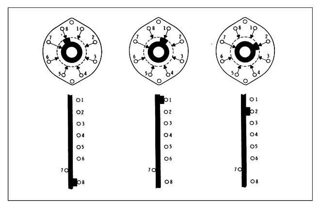
Figure 8-15. Three Positions of Index Light Selector Wafer
