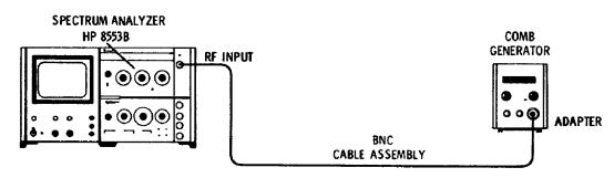
Figure 4-8. Tuning Dial Accuracy Test
