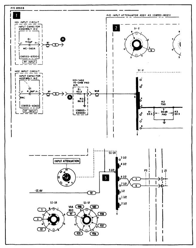
Figure 7-5. H01/H02 Schematic Changes for Service Sheet 3, Figure 8-26.
