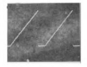
Oscilloscope: .2V/Div 5 msec/Div 10:1 probe <u>Analyzer</u>: PER DIVISION 2 msec/Div 10 MHz/Div
