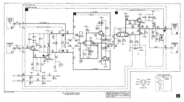
Figure 8-36. Automatic Phase Control and Sampler/Amplifier Circuits
