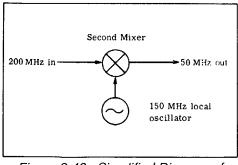
Figure 8-43. Simplified Diagram of Second Converter.
