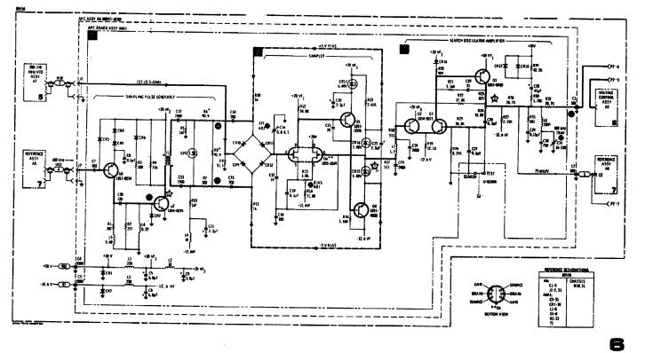
Figure 5. Automatic Phase Control and Sampler/Amplifier Circuits, Schematic Diagram (replacement for Service Sheet 6 in 8553B Operating and Service Manual)
