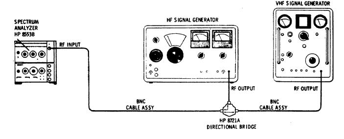
Figure 4-12. Intermodulation Distortion Test (ERRATA)
