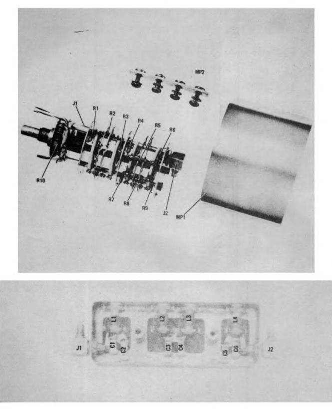
Figure 8-25. 120 MHz Low Pass Filter A11 (08553-6001) Component Locations
