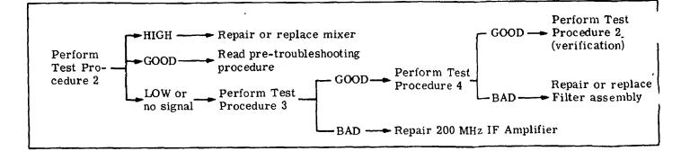
Simplified Test Procedure Tree
