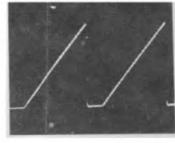
Oscilloscope: 5 msec/Div 0.2V/Div 10:1 probe
